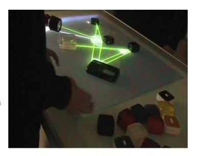
A LightTable, a purpose built 'tangible', was developed to explore how physical objects, reinforced with dynamic digital images to display invisible scientific phenomena, can support students' understanding of science. The LightTable helped students explore the behaviour of light with objects of different colours, shapes and textures, i.e. how light is reflected, refracted or absorbed with these different kinds of objects.
