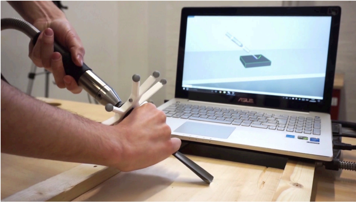
Figure 2. The gouges are mounted on a reciprocating electric tool and tracked with 3d printed MOCAP markers.
