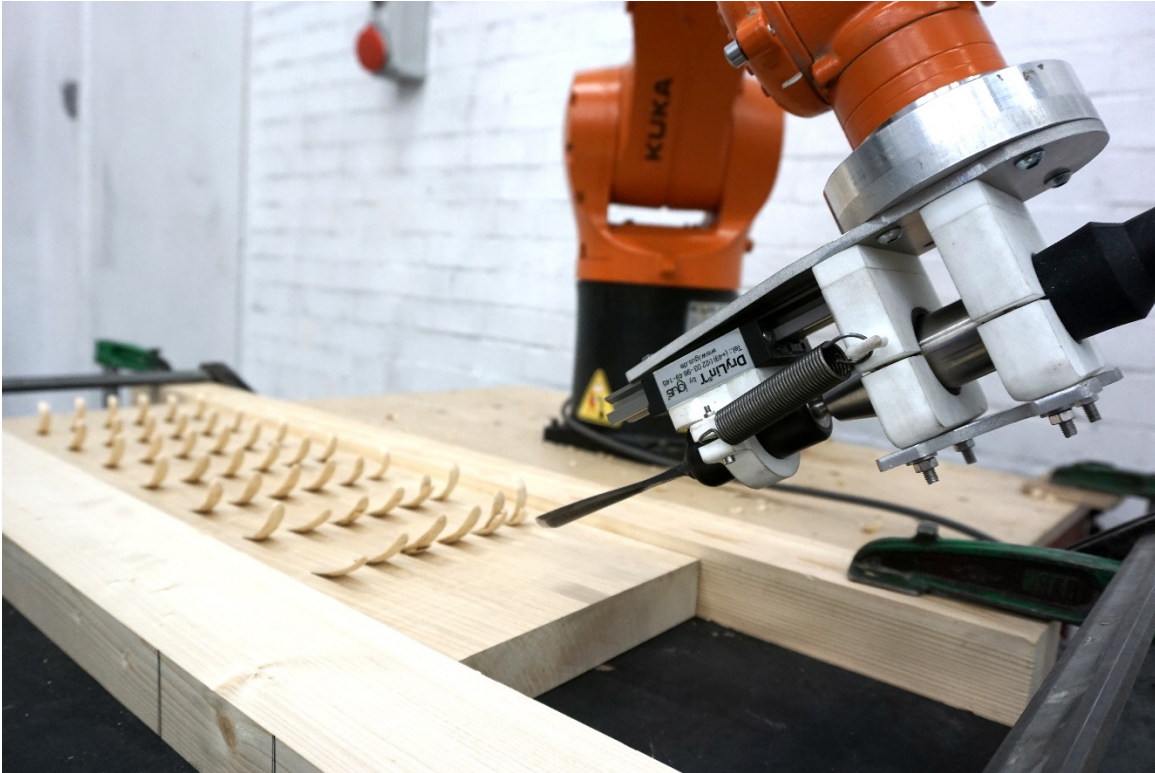
Figure 7. Based on the network trained with the information gathered by the human craftsman, robotic explorations of the narrowed-down parameter space are performed to increase the prediction abilities of the system.
