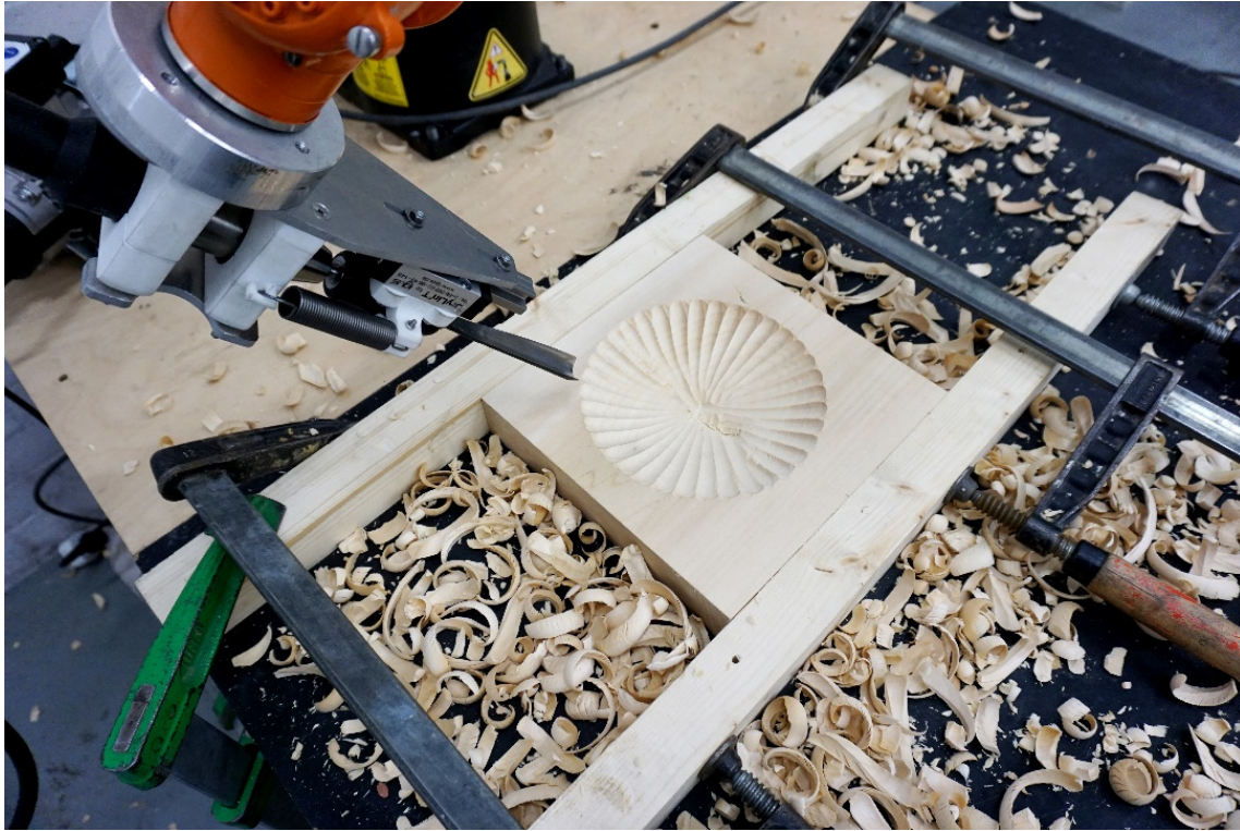
Figure 8. The trained networks are evaluated in the fabrication stage where they are required to provide the prediction of relevant fabrication parameters such as the tool angle variation or depth prediction of the cut itself.
