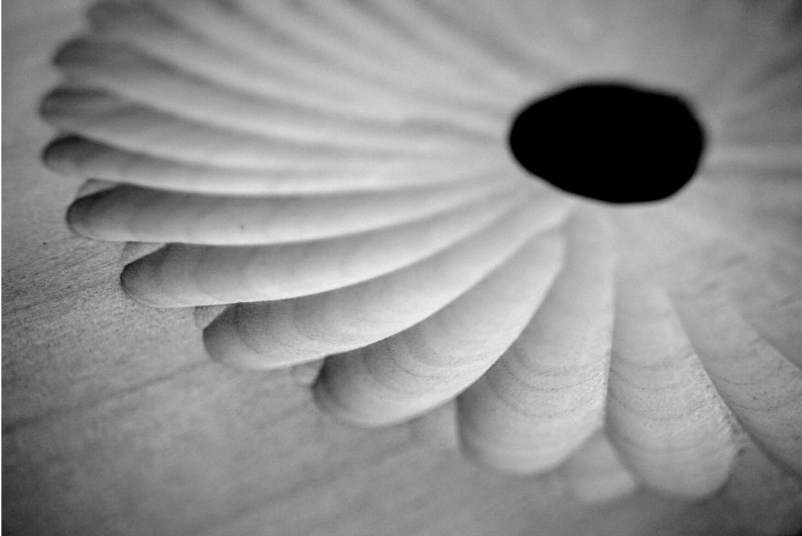
Figure 10. The carved circular patterns showed local deviations from the initial digital model due to the interaction between the cutting tool and local material properties such as the wood grain structure.
