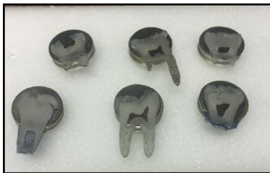
Figure 6-2: Image shows the six samples coated with gold- palladium layer and mounted on samples holder to be tested using SEM
