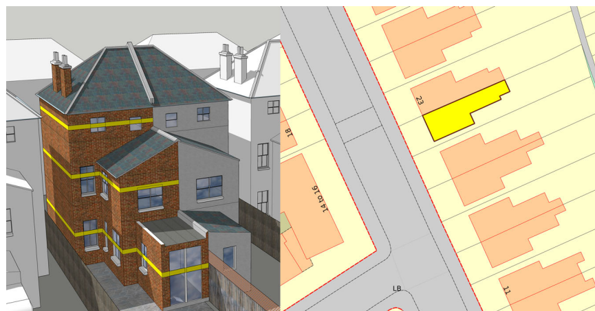
Figure 4. Storey area inference method applied to a fairly typical inner-London domestic building. Areas are calculated at the three levels marked by the yellow bands.
