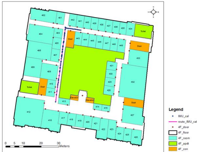
Fig. 6. Calibrated route and positions of each step event of PDR based positioning.
