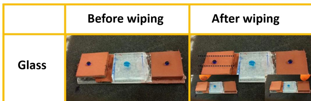
**Fig. 5.15** Finger-wipe tests on uncoated SH-Cu, plain and coated SH-Cu glass substrates, respectively (from left to right). The coating without PDMS was partly removed by a finger wipe while the superhydrophobic glass with PDMS coating sustained water proofing properties, indicating the coating becomes more robust.
