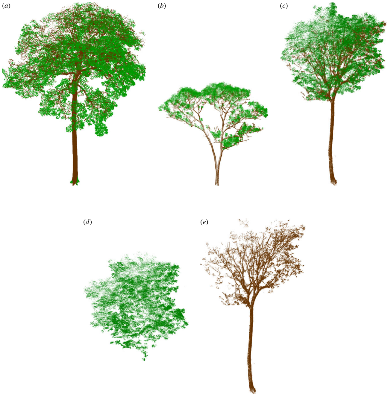
Figure 9. Examples of leaf/wood separation algorithm applied to trees of varying type, using the framework developed by Boni Vicari [82,83]. (a–c) A single ash tree from Wytham Woods [45,46]: (a) leaf and wood material; (b) leaf points only; (c) wood points only. (d,e) Individual trees with leaf (green) and wood (brown) material separated: (d) tropical hardwood (sp. unknown) from Nouragues, French Guiana [15]; (e) eucalypt ( Eucalyptus leucoxylon ), from Rushworth forest, Victoria, Australia [51].
