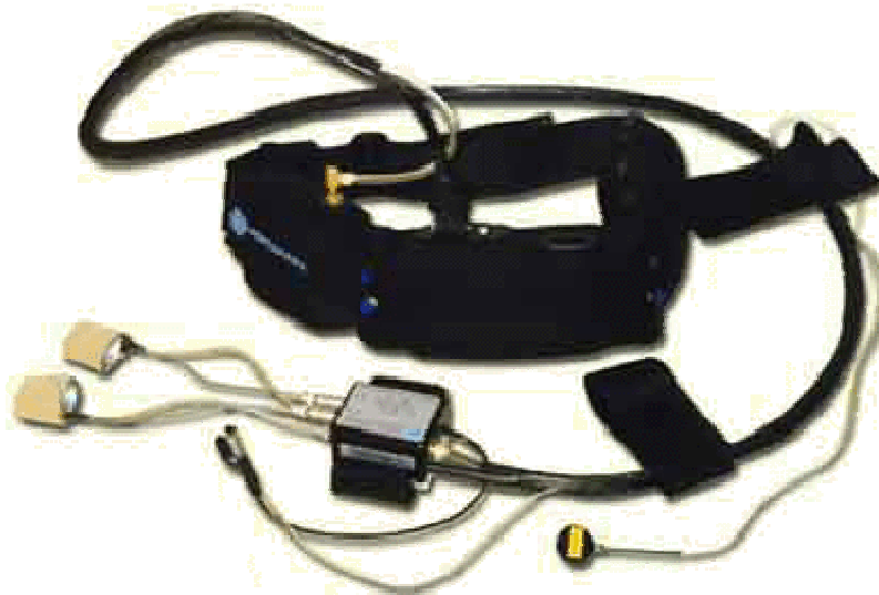
Figure 2:3 Portapres used for non-invasive beat-to-beat recording of cardiovascular indices. Two Velcro finger cuffs (bottom left) are shown connected to the fronted unit. Additional leads shown allow height correction to be performed prior to readings.
