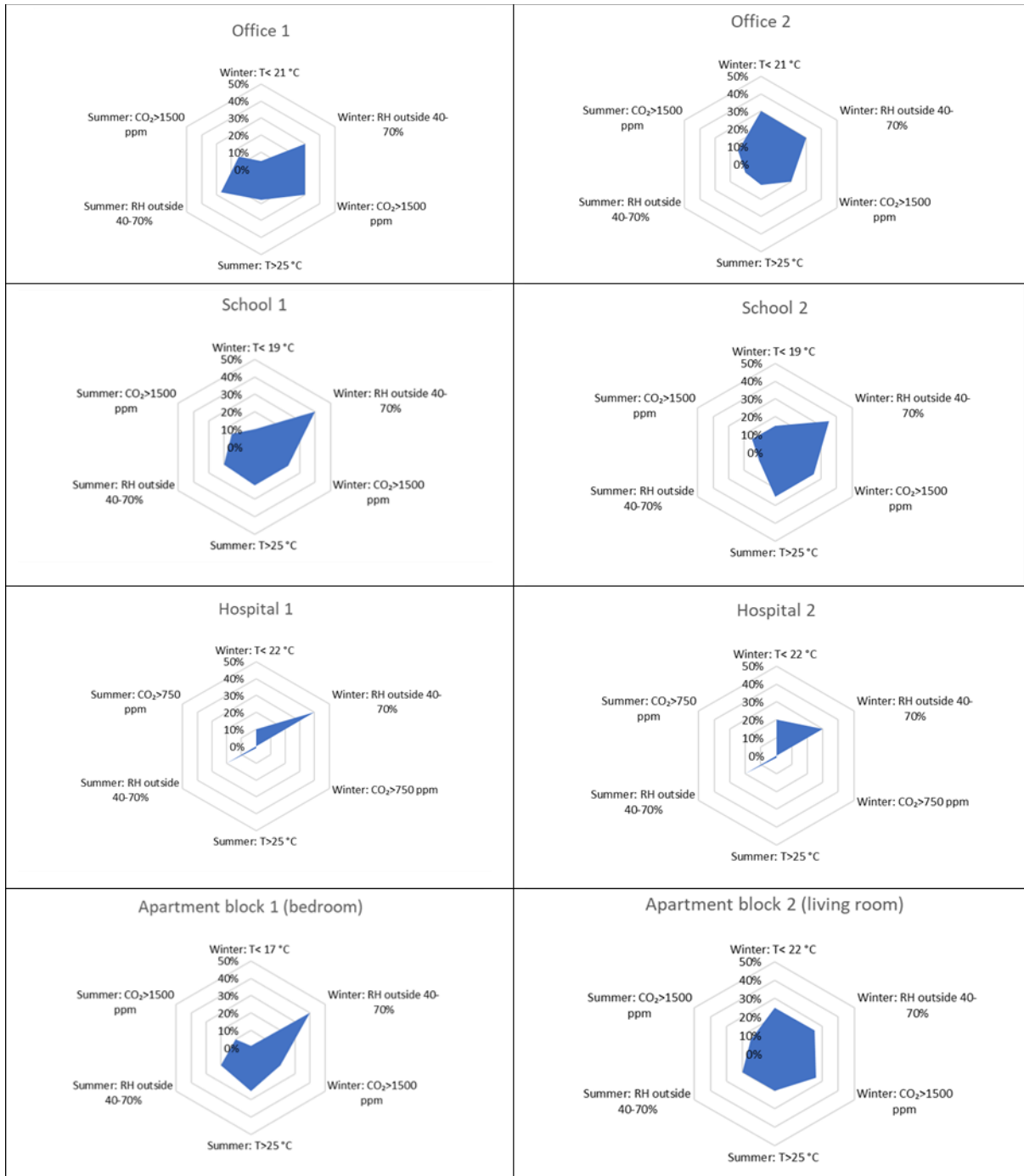
Figure 7 – The performance gap in thermal comfort and IAQ
