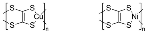
Figure 7. Molecular structures of two coordination polymers, containing Cu (p-type) or Ni (n-type). The counterions are omitted for clarity.
