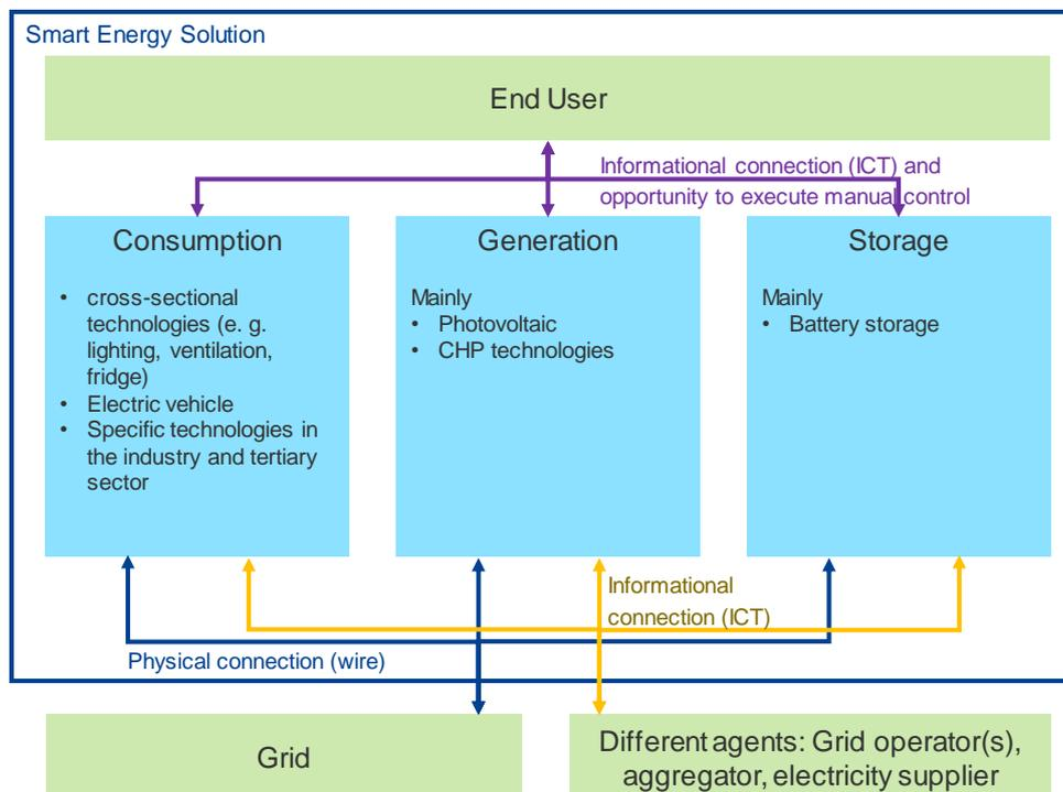
Figure 1 -Conceptual visualization of elements of a Smart Electricity Solution
