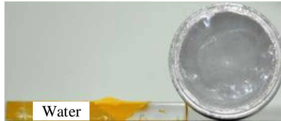
205 206 Fig 6. Surface topography of pmma specimen filled with water after freezing and 207 peeling the accumulated ice
