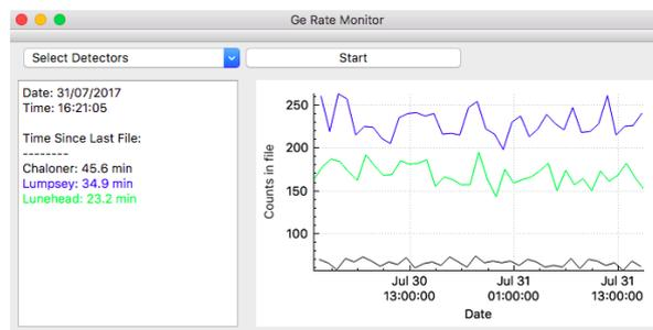
Figure 8: The GeMonitor software looking at data from the three detectors. The software allows users to monitor both count rates and the time since the last file was acquired. If the time goes significantly over an hour, operators are informed via instant messenger.
