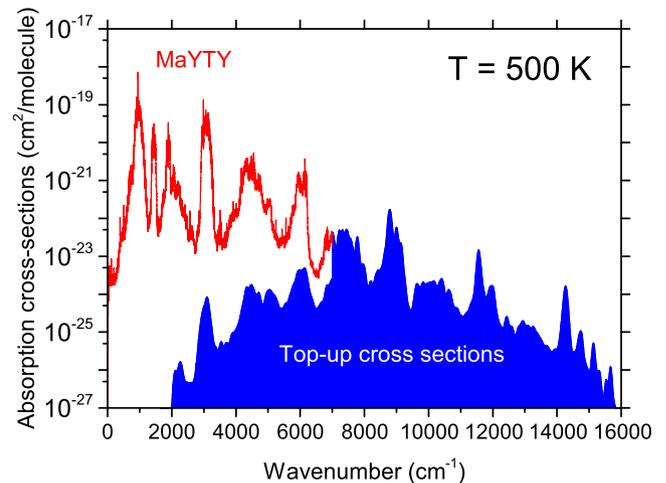
**Figure 11.** The vibrational ‘top-up’ cross-sections of  $\text{C}_2\text{H}_4$  computed using the vibrational line list with the three-band model at  $T = 500 \text{ K}$  (dark blue area) and the ro-vibrational intensities generated using the ExoMol line list with the Gaussian line profile of HWHM =  $1 \text{ cm}^{-1}$  (red line).
