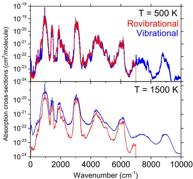
**Figure 10.** Comparing the ro-vibrational and vibrational intensities of  $\text{C}_2\text{H}_4$  at  $T = 500 \text{ K}$  and  $T = 1500 \text{ K}$ : The ‘ro-vibrational’ cross-sections of  $\text{C}_2\text{H}_4$  were computed using the MaYTY line list and the Gaussian line profile with HWHM =  $1 \text{ cm}^{-1}$ . The ‘vibrational’ cross-sections were computed using the vibrational line list with the normalized band profiles scheme (see text).
