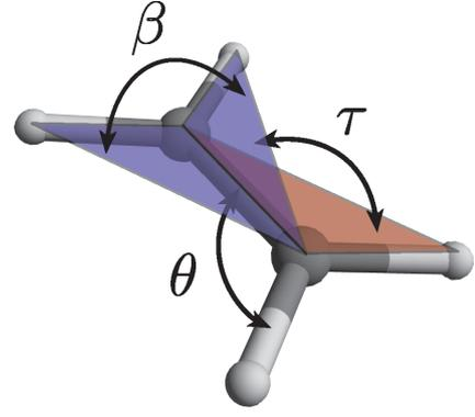
**Figure 1.** Definition of angular internal coordinates in ethylene.
