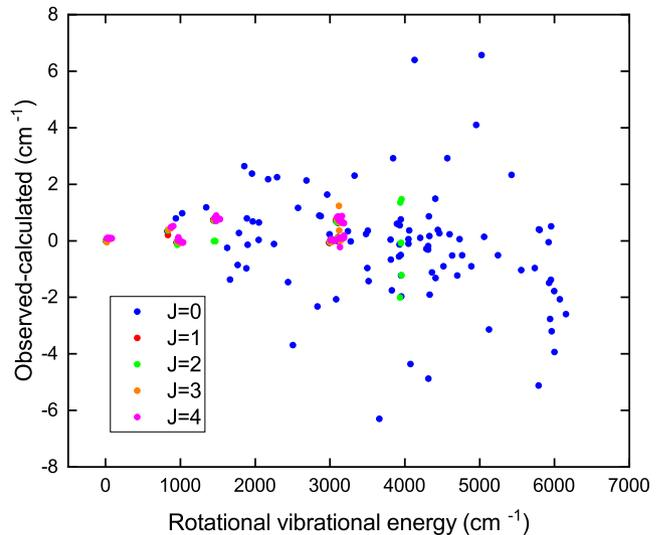
**Figure 2.** Observed–calculated rotational-vibrational energies after refinement. Vibrational energies (blue dots) with larger discrepancies were given a 1000 times smaller weighting in the refinement with respect to HITRAN vibrational energies.
