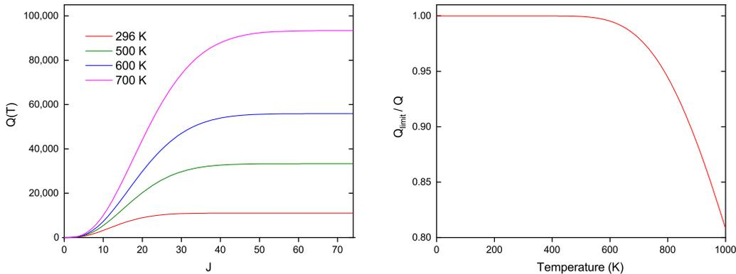
**Figure 4.** Partition functions of  $\text{C}_2\text{H}_4$ : Convergence of partition function  $Q(T)$  at different temperatures with respect to the rotational quantum number  $J$  (left) and  $Q_{\text{limit}}/Q$  as a function of temperature (right).
