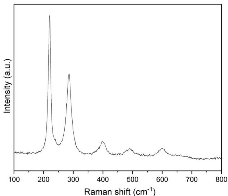
**Figure S4.** Strong bands for  $\text{Fe}_3\text{O}_4$ <sup>8</sup> detected using Raman spectroscopy of the film synthesized via “quenching” at 450 °C.
