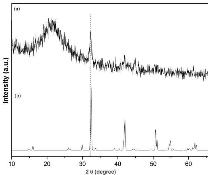
**Figure S1.** PXRD pattern of a  $\text{Fe}_{0.48}\text{TiSe}_2$  film (a) prepared by LPCVD of 1 at 1000 °C for 18h, followed by gradual cooling to room temperature. (b) XRD standard pattern for the  $\text{Fe}_{0.48}\text{TiSe}_2$  material, extracted from ICSD.<sup>7</sup> The pattern shows high fluorescence of iron with the copper beam from the anode on the X-Ray instrument.
