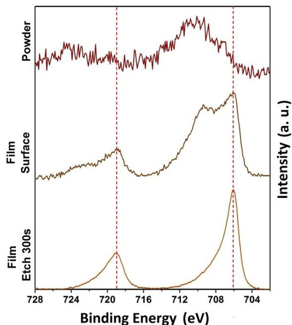
**Figure S2.** A visual change in the Fe XPS of the samples is apparent. It is highly likely that  $\text{Fe}_3\text{O}_4$  species is present both in the powder and in the surface of the thin film due to its exposure to air (main peak at BE = 710 eV). Upon XPS depth profile analysis in the thin film, inner layers (300 s etch) showed a Fe 2p environment at 706.7 eV and 719.2 eV.
