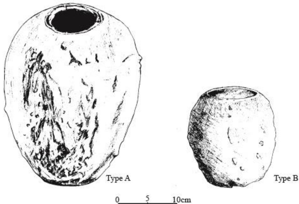
Figure 23. Schematic drawing of the recognized Ile-Ife glass crucible types, showing the difference in size. There is variation in the overall morphology of the crucible beyond what is represented in these drawings. The scale is estimated based on images in Willett (2004). (Drawing by Oluseyi Agbelusi).
