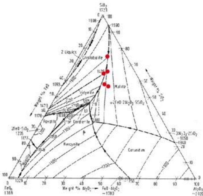
Figure 19b. Projection of the composition of Ile-Ife domestic pottery (red circles) into the ternary phase diagram for ferruginous ceramic. The composition falls near a cotectic trough indicating relatively low theoretical melting temperatures. Actual melting temperatures would be even lower due to the presence of minor oxides such as potash and others working as fluxes.
