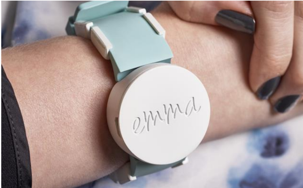
Figure 7.1.1.1. The Emma watch delivers high frequency of vibration at 200 Hz through six small devices, three on each side of the wrist.
