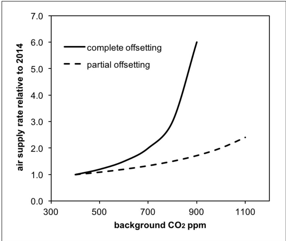
Figure 3. Two strategies for offsetting effects of increases in background CO<sub>2</sub> concentration on indoor CO<sub>2</sub> concentrations. The trajectory for complete offsetting has an asymptote at 1000 ppm, and has been truncated at 900 ppm. The partial offsetting strategy in this example assumes that half of the increase in background CO<sub>2</sub> is offset by larger air flows.
