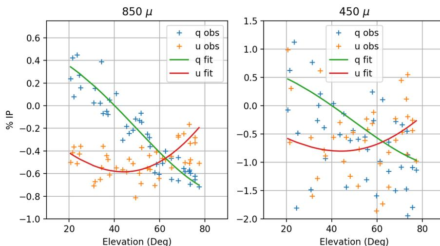
Figure 3. Measured IP and the best fitted model without the wind blind in place. Left : q and u data for 850  $\mu\text{m}$  and the fit to the 850  $\mu\text{m}$  data. Right: q and u data for 450  $\mu\text{m}$  and a scaled version of the 850  $\mu\text{m}$  fit. Note that the intensity scale for the 450  $\mu\text{m}$  plot is not the same as for the 850  $\mu\text{m}$  plot.
