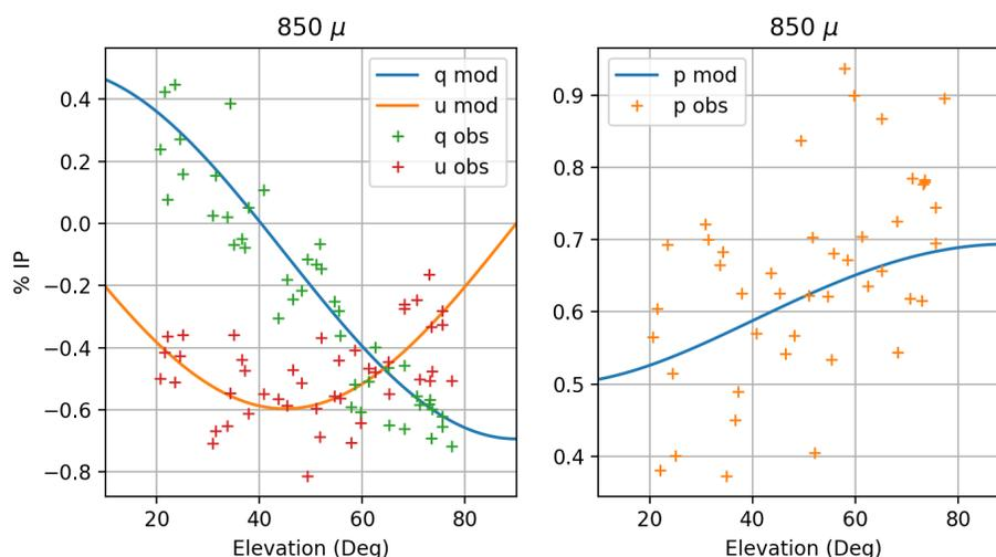
Figure 6. Comparison between the data and the model for IP generated by the six relay mirrors without the wind blind. (right) Observed (obs) and theoretical model (mod) for q and u. (right) Observed (obs) and theoretical model (obs) for degree of polarization. As predicted the degree of polarization is highest when the telescope points to zenith and decreases towards the horizon.
