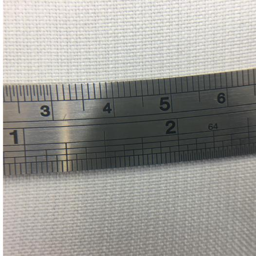
Figure 2. Close up image of a spare sample of wind blind material. Some optical optical distortion is apparent from the curvature of the ruler. The top scale on the ruler is in mm, bottom inches. As two threads being used together, the apparent thread pattern is  $\sim 500 \mu\text{m}$  instead of  $\sim 250 \mu\text{m}$ . Counting threads, the weave appears asymmetric in thread count of about 2% in the two directions.
