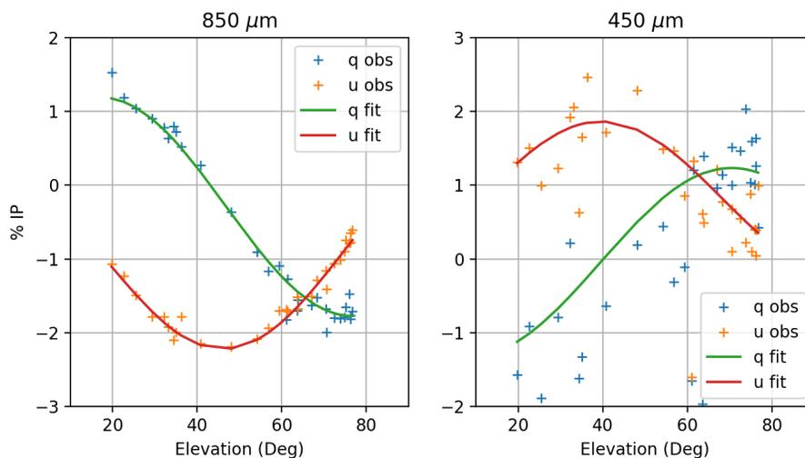
Figure 4. Measured IP with the wind blind in place. Left: Normalized Q and U data for 850  $\mu\text{m}$  and the fit to the 850  $\mu\text{m}$  data. Right: Normalized Q and U data for 450  $\mu\text{m}$  and the fit to the 450  $\mu\text{m}$  data. The IP is rotated about 90 degrees between the 850 and 450  $\mu\text{m}$  focal planes.
