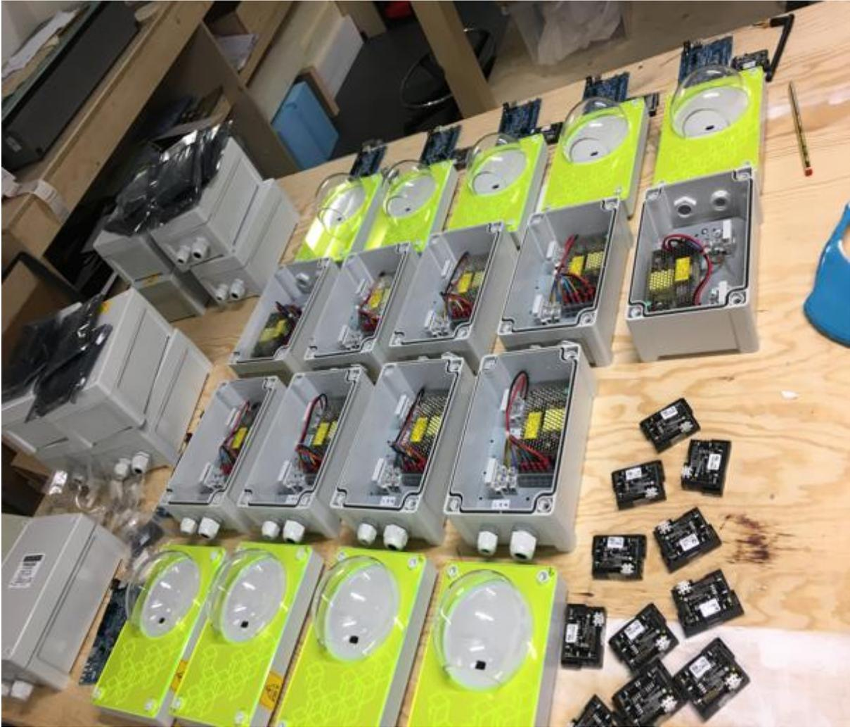
**Figure 4** ICRI Environmental Sensor Assemblies.
