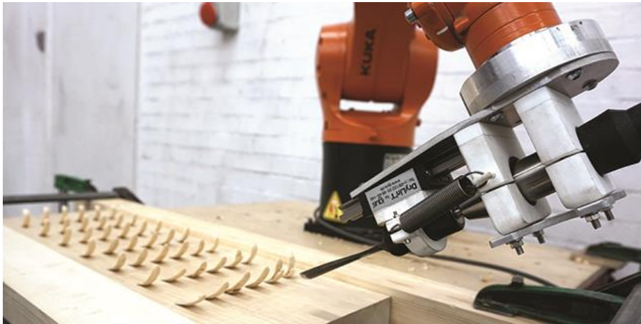
Fig. 4. The robotic training sessions allow to perform an in-depth exploration of selected parameters domain through a collection of finely interpolated cuts.
