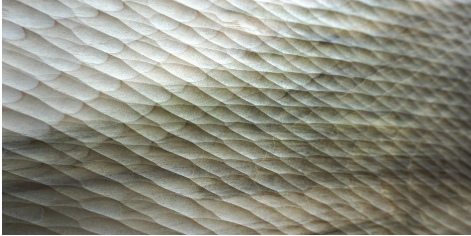
Fig. 11. Combining together prediction of cuts with different fabrication parameters, it's possible to simulate the final carved geometry in several pattern configurations.
