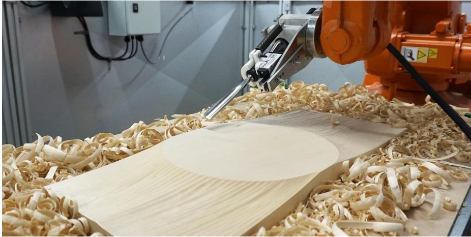
Fig. 6. In the robotic fabrication stage, the trained network is used to inform the robotic toolpath to carve the previously simulated geometries.
