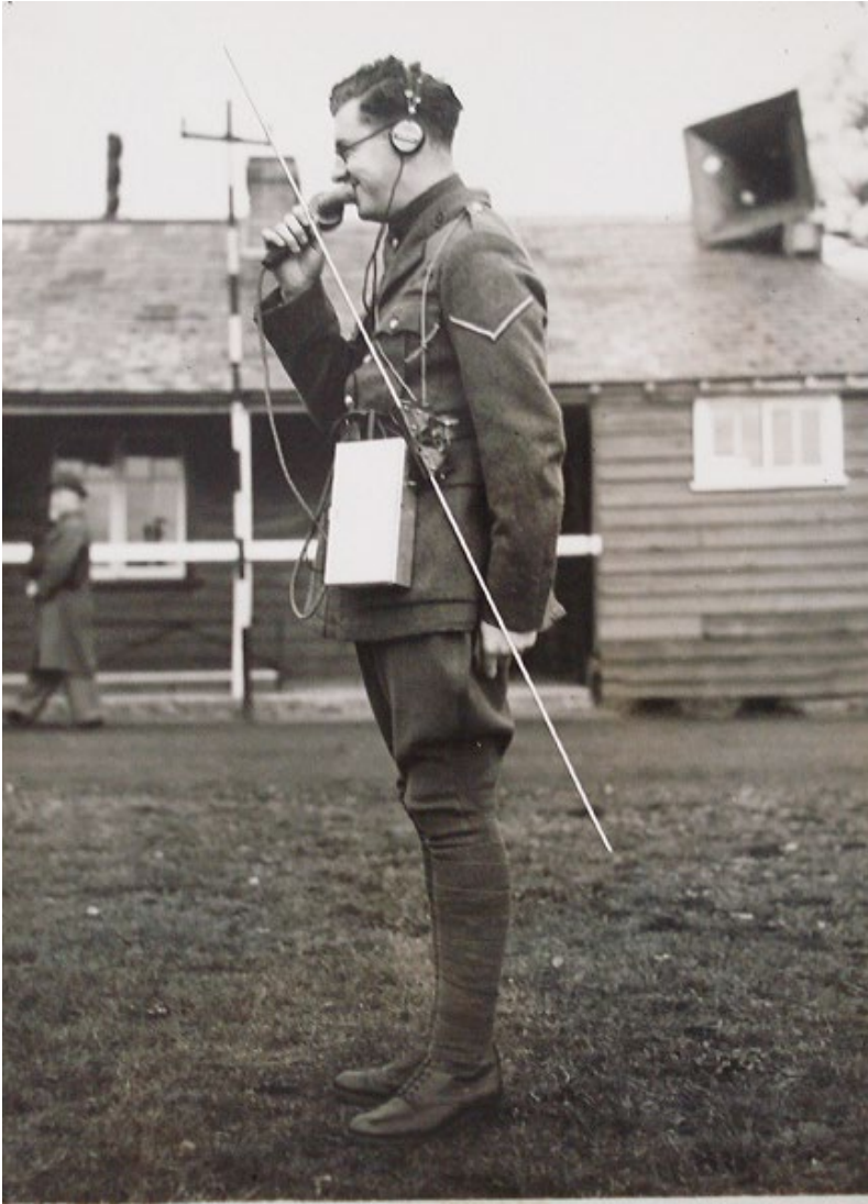
Fig. 11.2 A member of the CUOTC Signals Section – probably John Kendrew – using the duplex radio-telephony set developed by Ben Lewis, c.1937.
