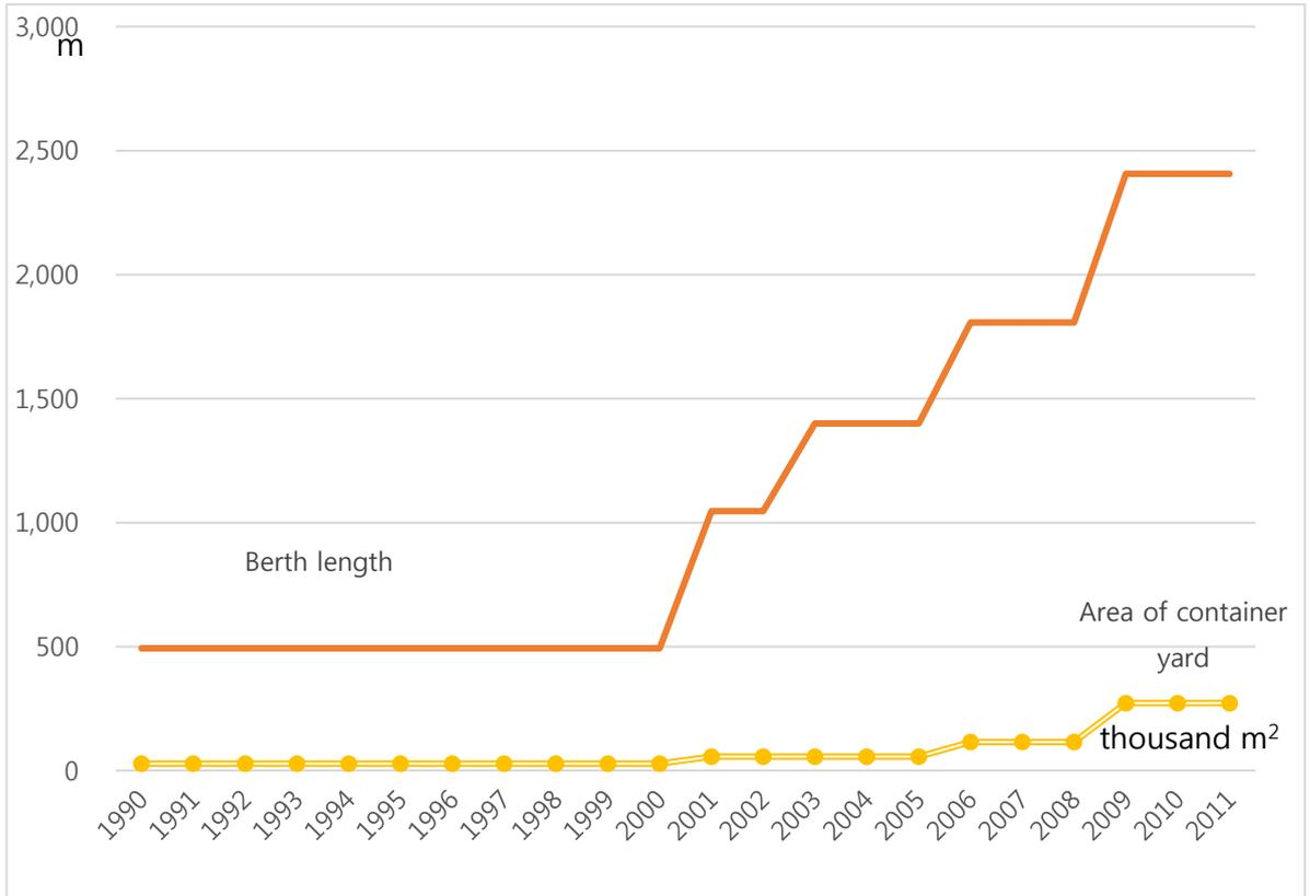
Figure 3.6: Berth length and area of container yards of Incheon Port
