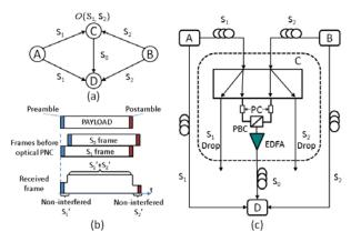
Fig. 2. (a) Example network utilizing network coding. (b) Frames before and after network coding. (c) Proposed optical PNC implementation.
