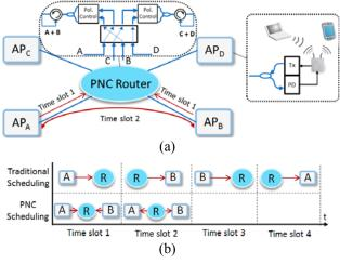
Fig. 3. (a) Proposed system architecture. (b) Comparison of the scheduling approach
