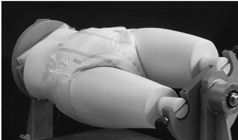
**Fig 3:** Equipment for measuring the absorption before leakage (ABL) of products.
