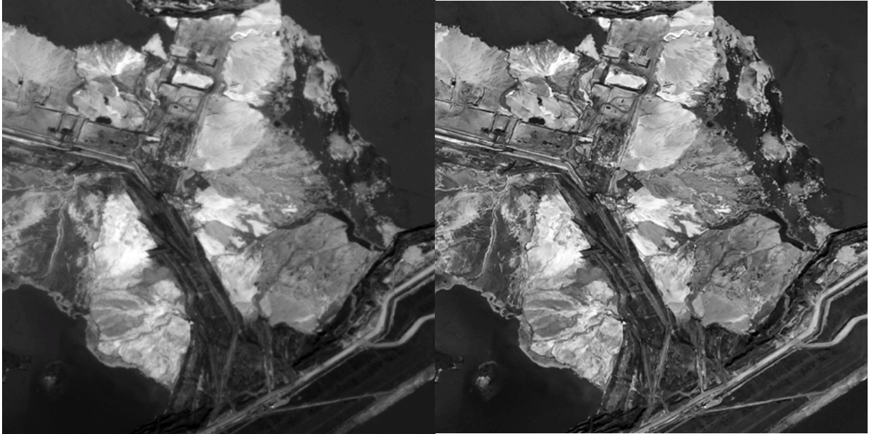
Figure 10. An example of a cropped sample of Deimos-2 4m MS green band image (DE2_11542_DE03; left) and 2m GAN single image SRR result (right).
