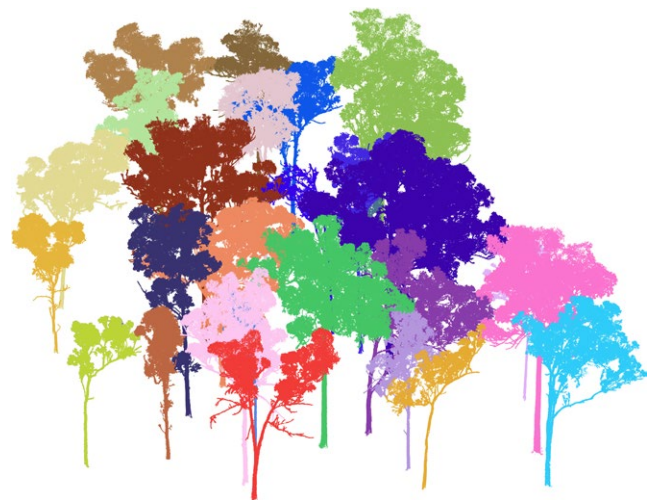
FIGURE 6 The 28 tree-level point clouds extracted from the KARA-001 ( Eucalyptus spp. open forest) larger-area point cloud via treeseq
