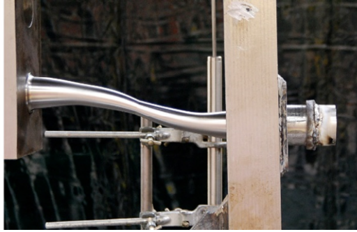
Fig. 8. Axial elongation of SSP2 after 30 cycles under CA = 7u_y
