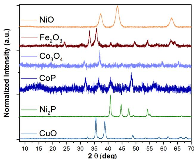
**Figure 1:** Powder X-ray diffraction patterns of MOF-derived NiO, Fe<sub>2</sub>O<sub>3</sub>, Co<sub>3</sub>O<sub>4</sub>, CoP, Ni<sub>2</sub>P and CuO NPs.
