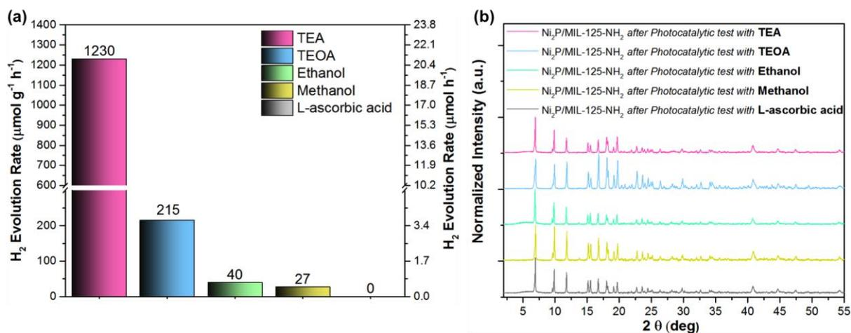
**Figure 5:** (a) Comparison of H<sub>2</sub> evolution rates of 9.2 wt% Ni<sub>2</sub>P/MIL-125-NH<sub>2</sub> with different electron donors, under visible light irradiation for 8 h, (b) Powder x-ray diffraction patterns of 9.2 wt% Ni<sub>2</sub>P/MIL-125-NH<sub>2</sub> after the photocatalytic test with different electron donors.
