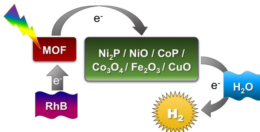
**Scheme 1:** Schematic representation of the strategy followed in this work: Step 1: use of different co-catalysts, Step 2: variation of the electron donors and Step 3: replacement of the electron donor with Rhodamine B (RhB), a dye that is used as a simulant organic pollutant.
