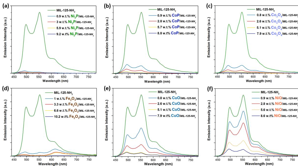
**Figure 4:** PL spectra of the suspensions of MIL-125-NH<sub>2</sub> with different amounts of: (a) Ni<sub>2</sub>P, (b) CoP, (c) Co<sub>3</sub>O<sub>4</sub>, (d) Fe<sub>2</sub>O<sub>3</sub>, (e) CuO and (f) NiO. The co-catalyst-induced quench in the PL follows the descending order of Ni<sub>2</sub>P > CoP ≈ Co<sub>3</sub>O<sub>4</sub> > Fe<sub>2</sub>O<sub>3</sub> > CuO > NiO. The excitation wavelength was 420 nm.
