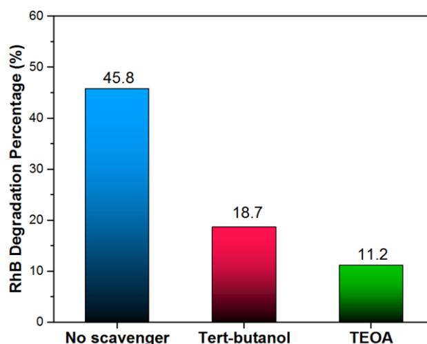
**Figure 7:** The impact of the incorporation of TEOA as hole scavenger, tert-butanol as •OH radical scavenger, or no scavenger on the RhB degradation rate after 3 h photocatalytic test.
