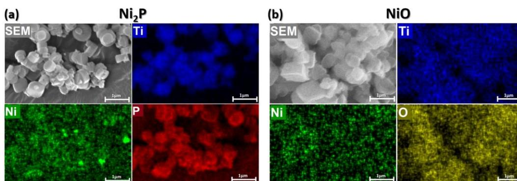
**Figure 3:** (a) SEM image of Ni<sub>2</sub>P/MIL-125-NH<sub>2</sub> after 8-hour photocatalytic test and the corresponding EDX maps of Titanium, Nickel and Phosphorus and (b) SEM image of NiO/MIL-125-NH<sub>2</sub> after 8-hour photocatalytic test and the corresponding EDX maps of Titanium, Nickel and Oxygen. Scale bar: 1 μm.
