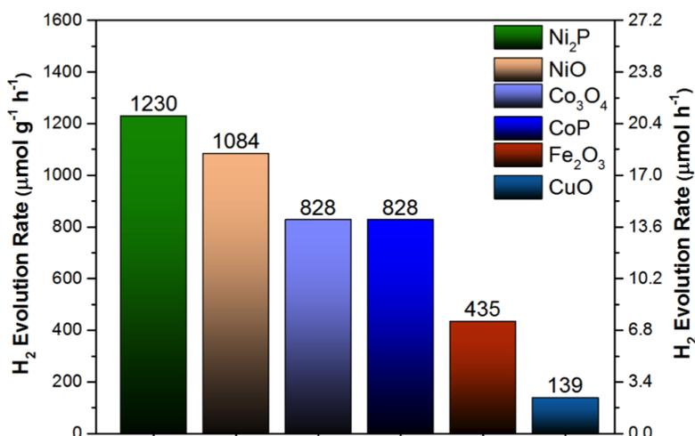
**Figure 2:** Comparison of H<sub>2</sub> evolution rates (with respect to MIL-125-NH<sub>2</sub>) of 9.2 wt% Ni<sub>2</sub>P/MIL-125-NH<sub>2</sub>, 8.6 wt% NiO/MIL-125-NH<sub>2</sub>, 7.9 wt% Co<sub>3</sub>O<sub>4</sub>/MIL-125-NH<sub>2</sub>, 8.8 wt% CoP/MIL-125-NH<sub>2</sub>, 10.2 wt% Fe<sub>2</sub>O<sub>3</sub>/MIL-125-NH<sub>2</sub> and 7.9 wt% CuO/MIL-125-NH<sub>2</sub> under visible light irradiation for 8 hours.
