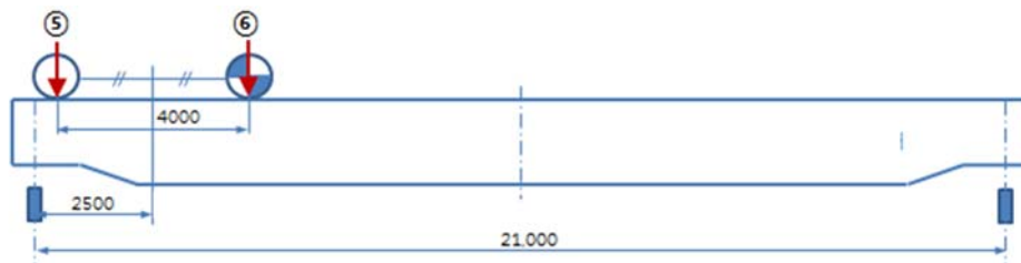
(b) Loading position 2: The trolley locates at end of the auxiliary girder
