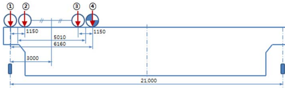
(b) Loading position 2: The trolley locates at end of the main girder
