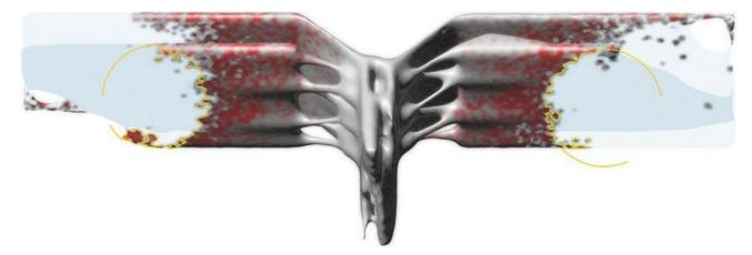
Interior view of the multi-material mullion interface showing the aluminium (silver), alumina (red), and glass (translucent blue) sub-material distribution. Credit: Kostas Grigoriadis
