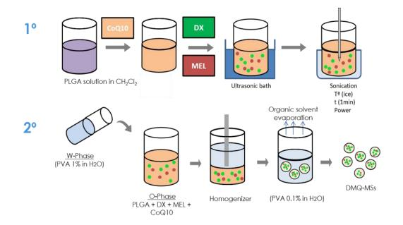
Figure 1. Elaboration process of the mullti-loaded MSs.
