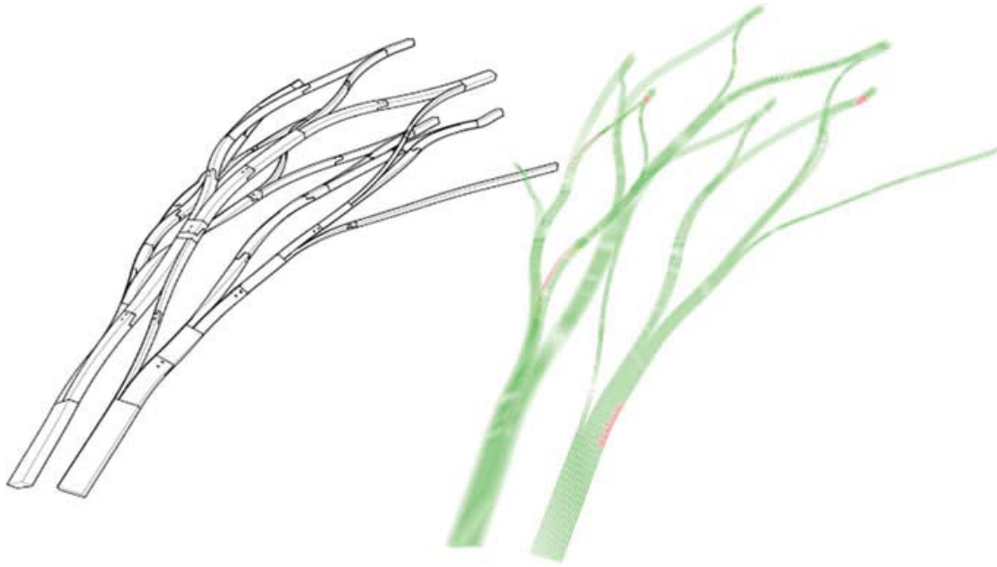
Fig. 4. The area around a foot condition extracted from the global design proposal, showing both geometric information from the beam model ( left ) and material information from the material model ( right ). In this case, the model is checked to see if the constituent lamellas of each module are within their bending limits
