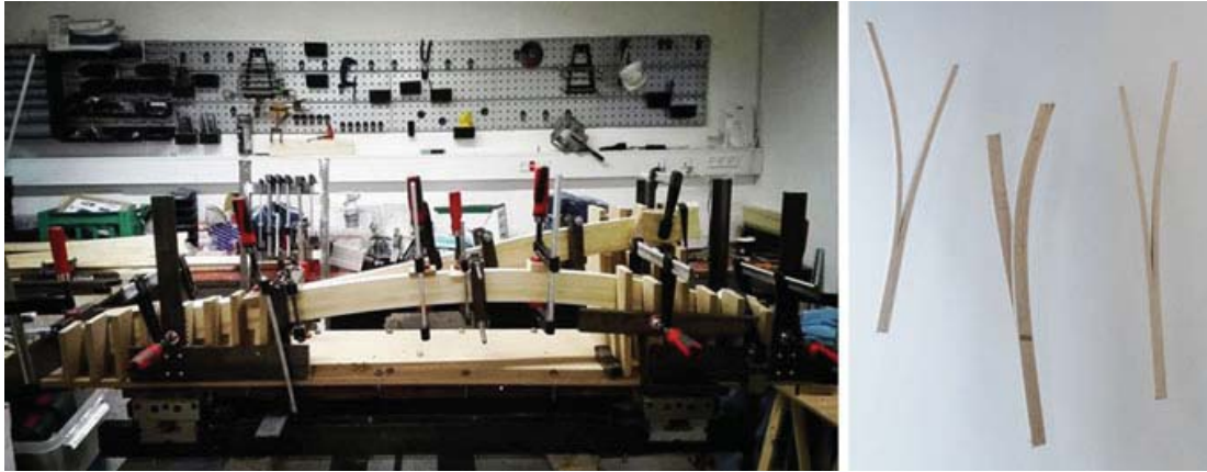
Fig. 7. Forming one of the bifurcating glulam components ( left ) and some finished examples ( right )
