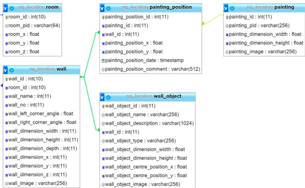
Figure 7. The database tables structure and the relationships formed for storing the NG location data. Simple width and height values are stored in centimetres and the various x, y and z dimensions can be defined as absolute values of latitude, longitude and altitude or as simple values relative to a local zero point for a given institution or location. A graphical representation of the possible absolute and relative positions relating to the location of a painting on a wall can be seen in Figure 8.
