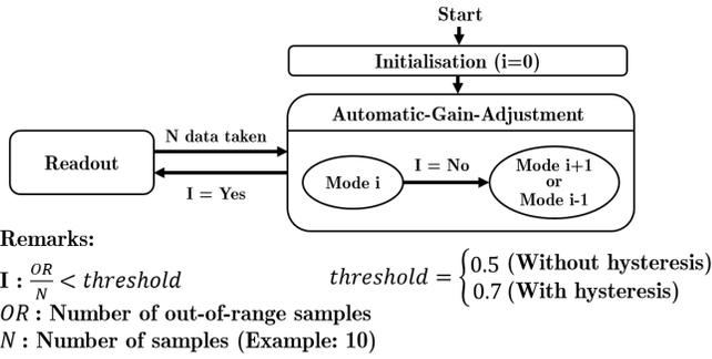
Fig. 3: The state diagram for autonomous gain control.
