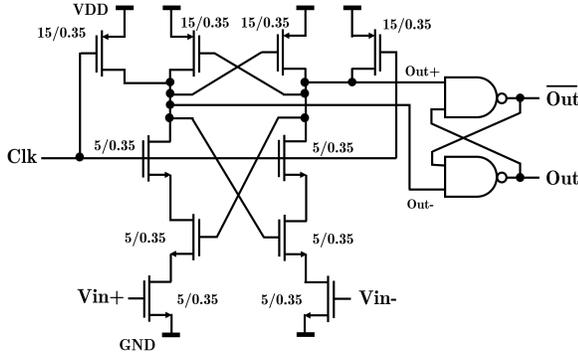
Fig. 4: The schematic of the clocked comparator.
