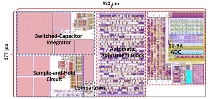
Fig. 5: Complete system layout with annotated floorplan
