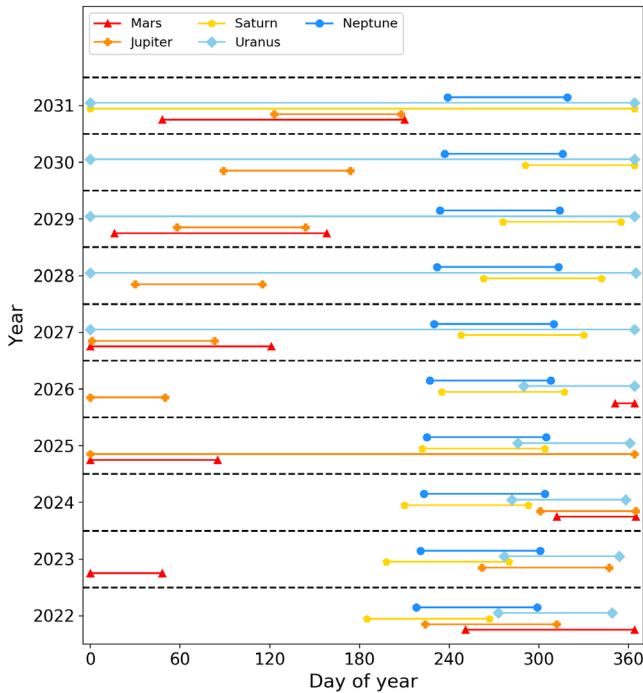
Fig. 7 Periods for which the outer planets lie within Twinkle’s field of regard from January 1, 2022, to January 1, 2032. Owing to Mars’s close proximity to Earth and Twinkle’s field of regard, Mars is only observable every other year.
