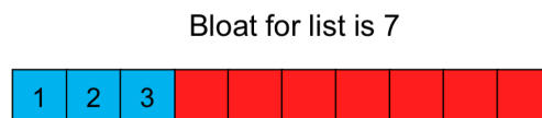
Figure 2.6: When an ArrayList is used with default parameters, it allocates memory for 10 entries.
