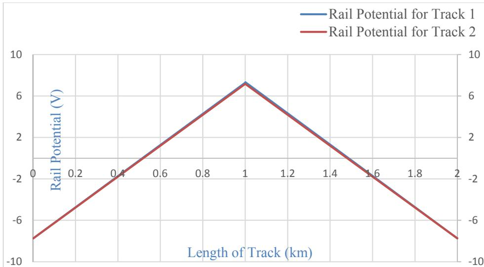
**Figure 53: Effect of Cross Bonding at Centre of the Track on Rail Potential**
