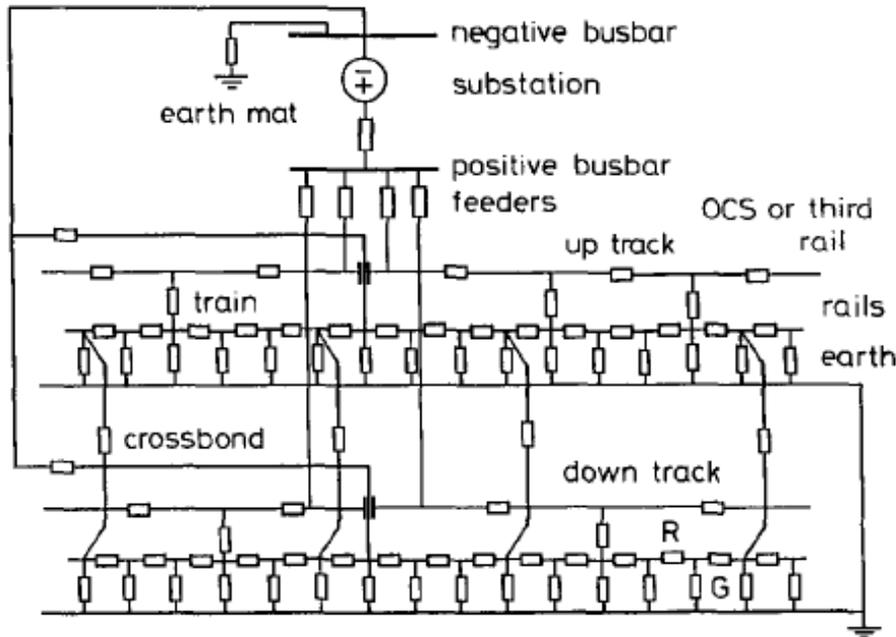
**Figure 13: Multi-ladder network representation of double-track [73]**
