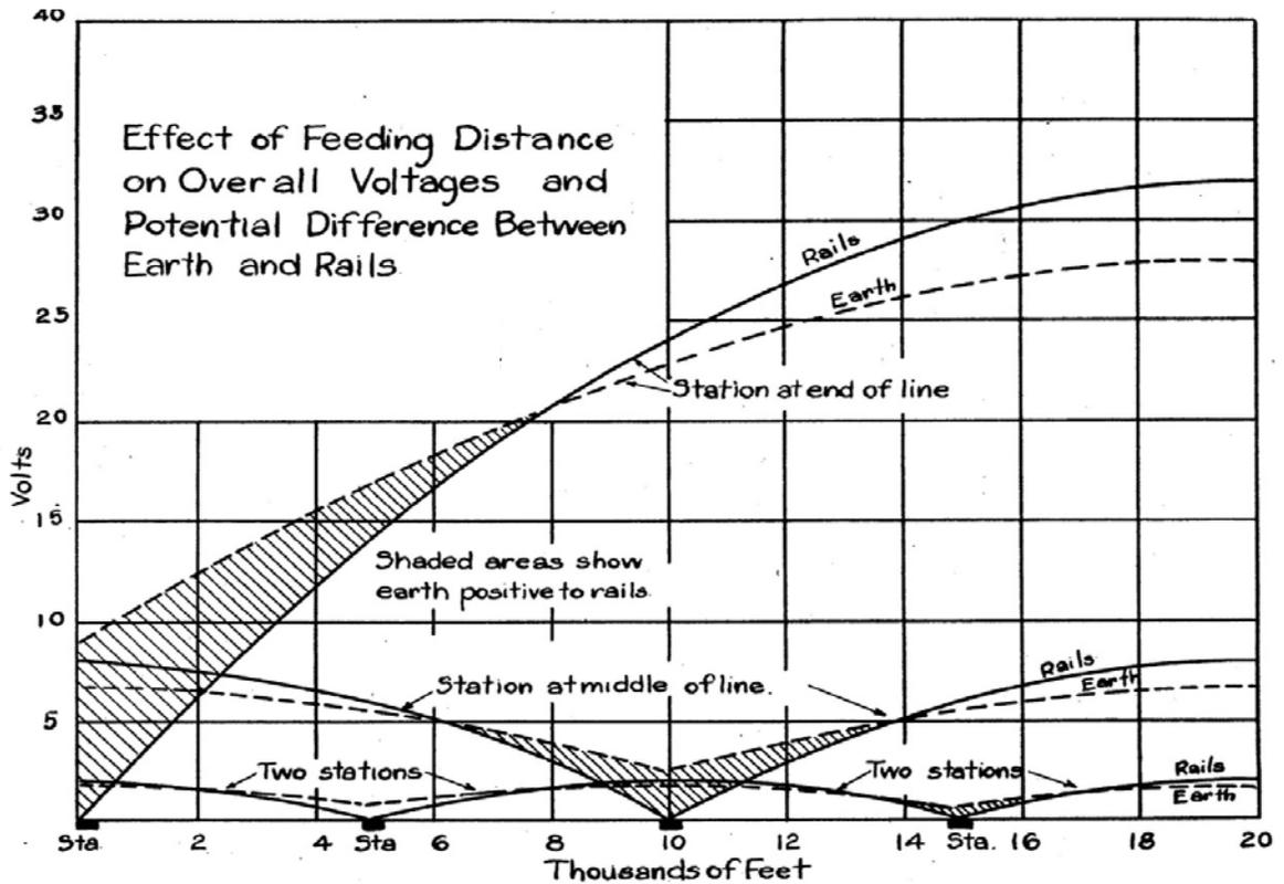
Figure 8: Effect of Substation Spacing on Voltage [1]
