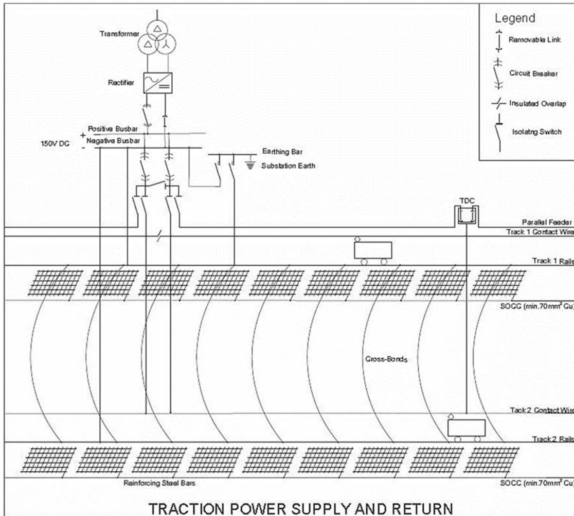
**Figure 57: Typical Parallel Track Traction Power Supply and Return Circuit**
