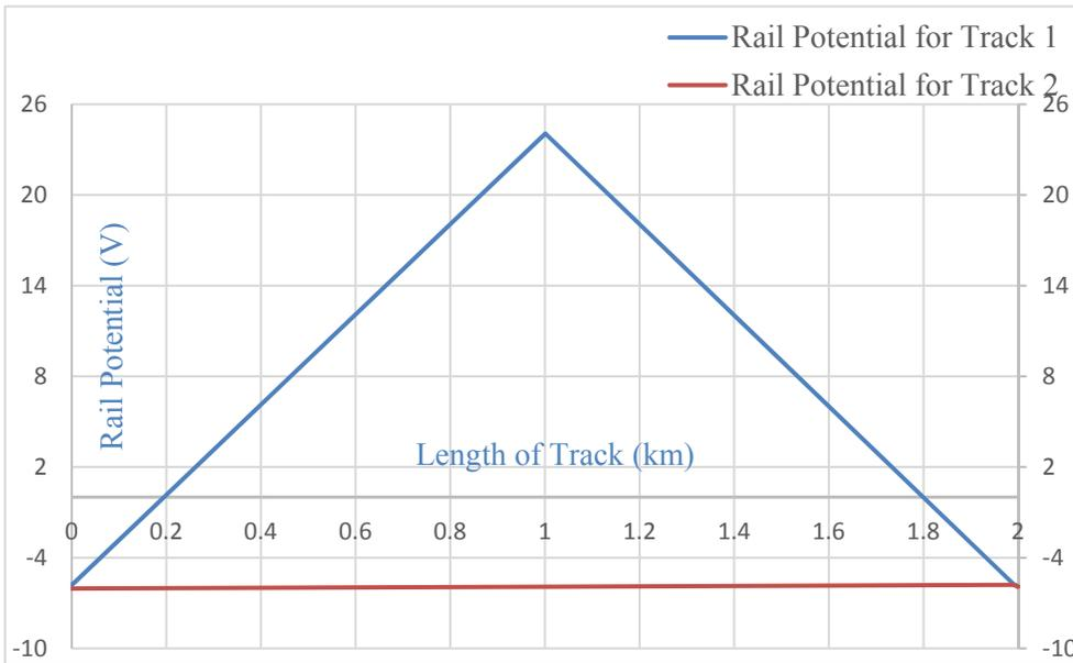
**Figure 52: Effect of no Cross Bonding on Rail Potential for Floating System**
