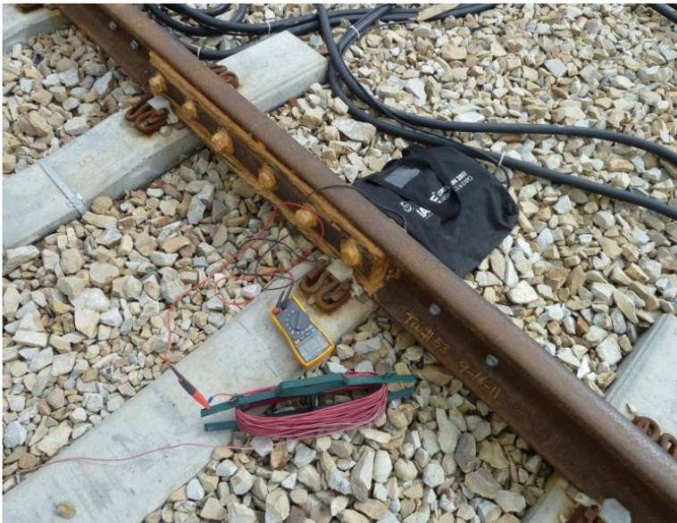
**Figure 37: Track-to-Earth Measurement – Ballasted Track**
