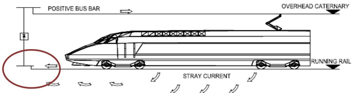
**Figure 4: Ungrounded / Floating System**
