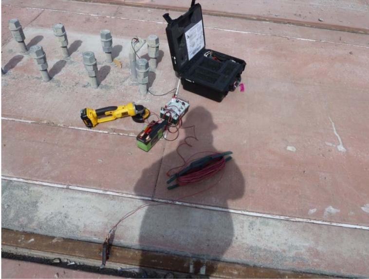
**Figure 40: Audio Frequency Test Setup**
