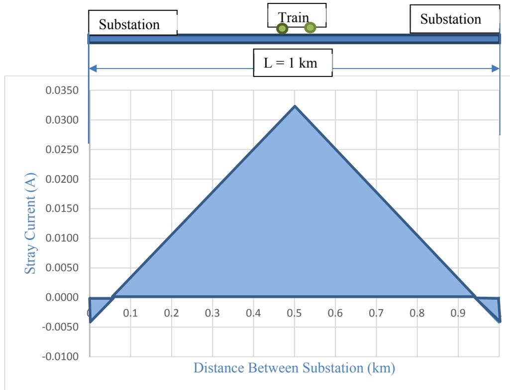
**Figure 49: Stray Current Model – Numerical Validation for Floating System**
