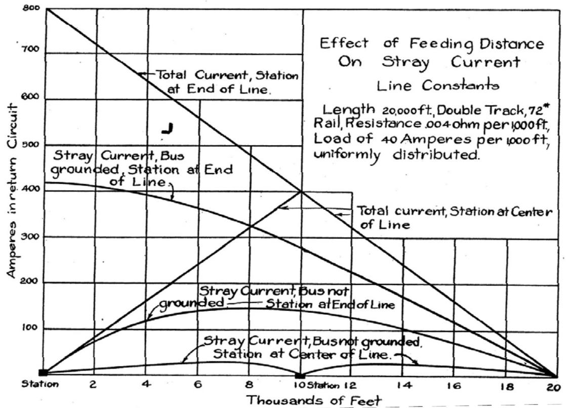
Figure 7: Effect of Substation Spacing on Stray Current [1]
