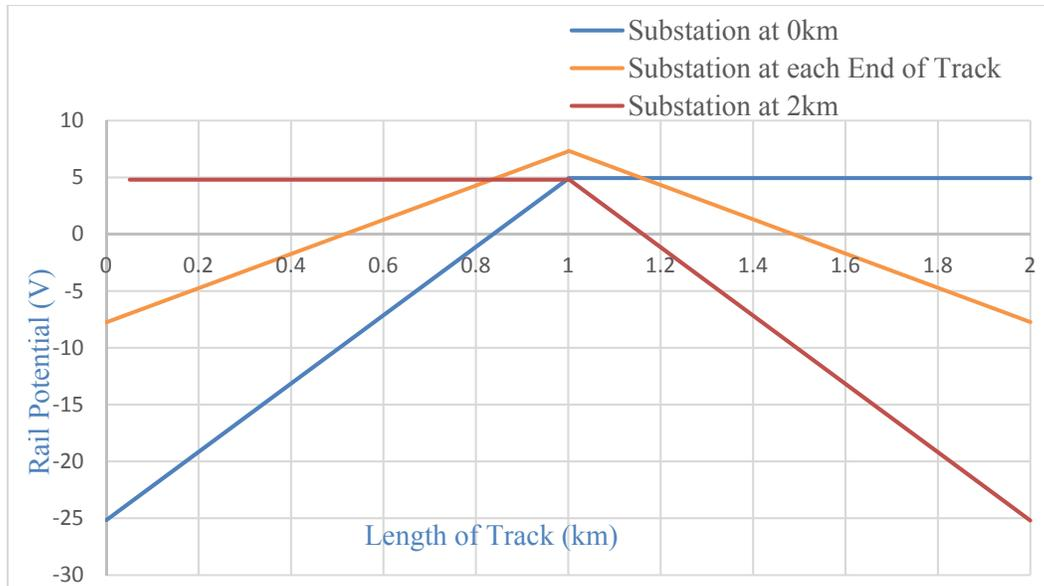
**Figure 50: Effect of Substation Location on Rail Potential in Floating System**
