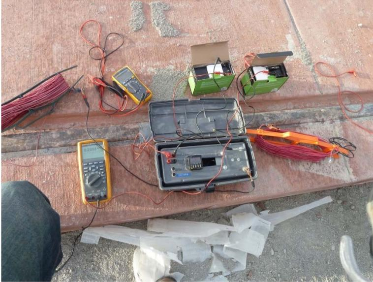
**Figure 36: Fluke Model 289 and 116 – Embedded Track Section**
