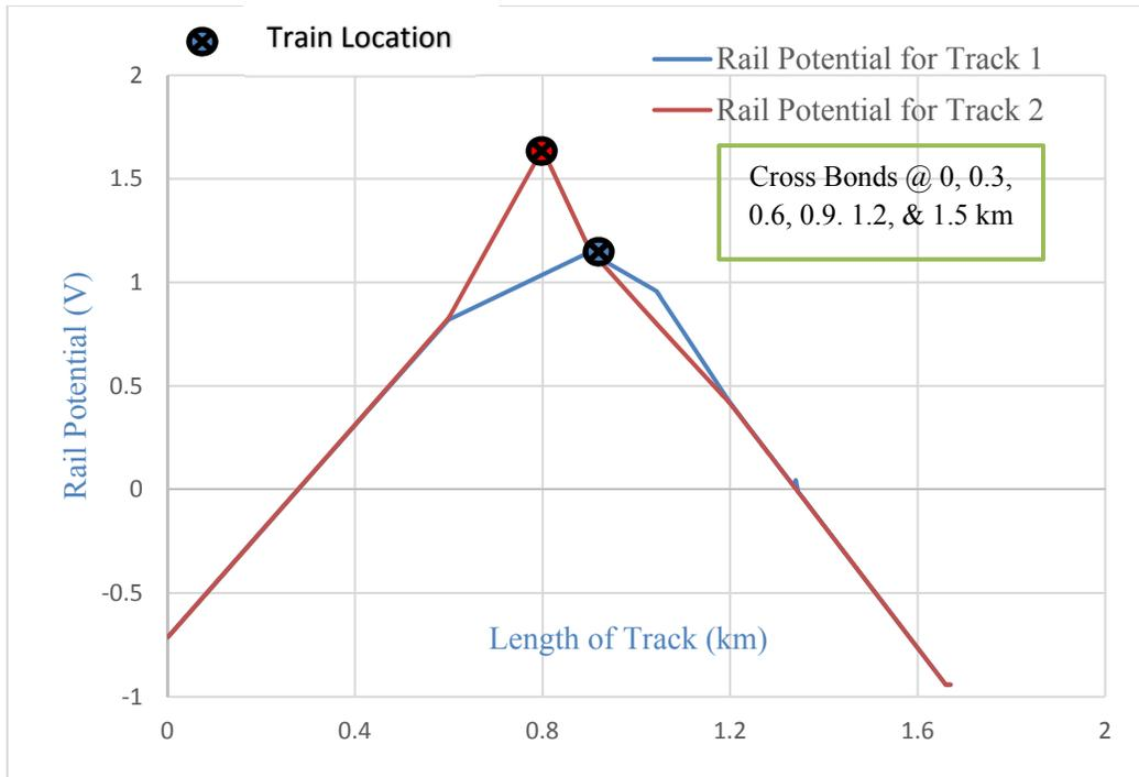
**Figure 58: Rail Potential for Two Track Transit System with Cross Bonding**
