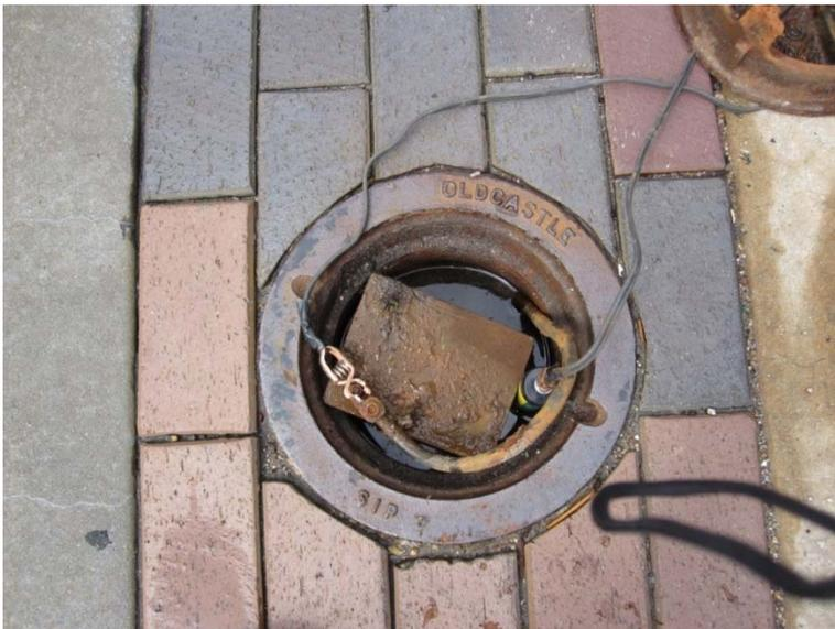
**Figure 32: Pipe to Soil Testing Location**
