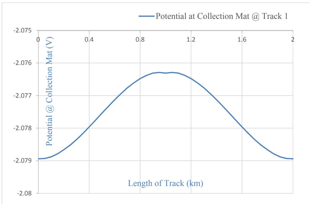
**Figure 55: Potential on Collection Mat with Cross Bonding**
