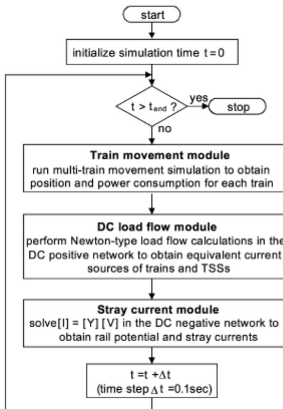
**Figure 15: Computer simulation Flowchart for Stray Current [30]**
