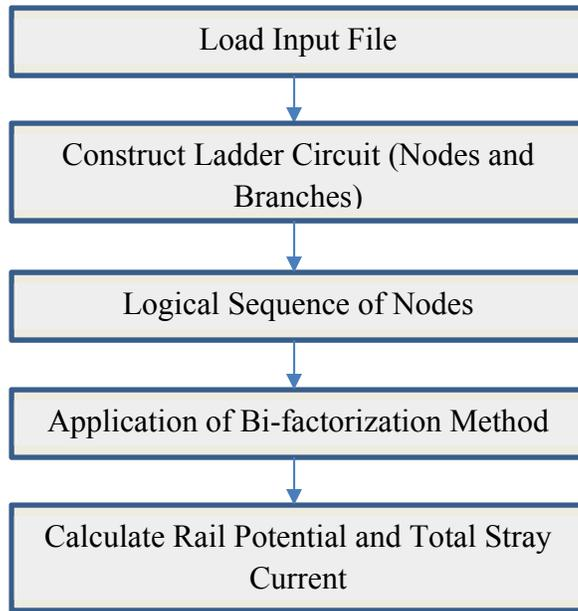
**Figure 48: Logical Sequence of the Modelling Process**
