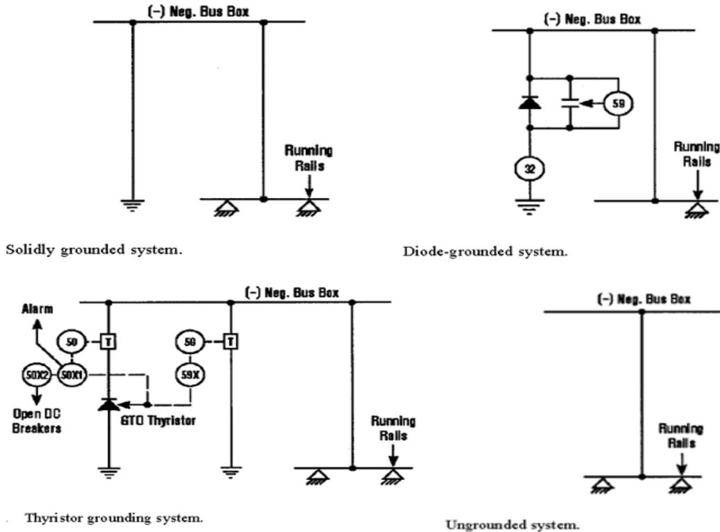
Figure 6: Grounding Systems Types [22]
