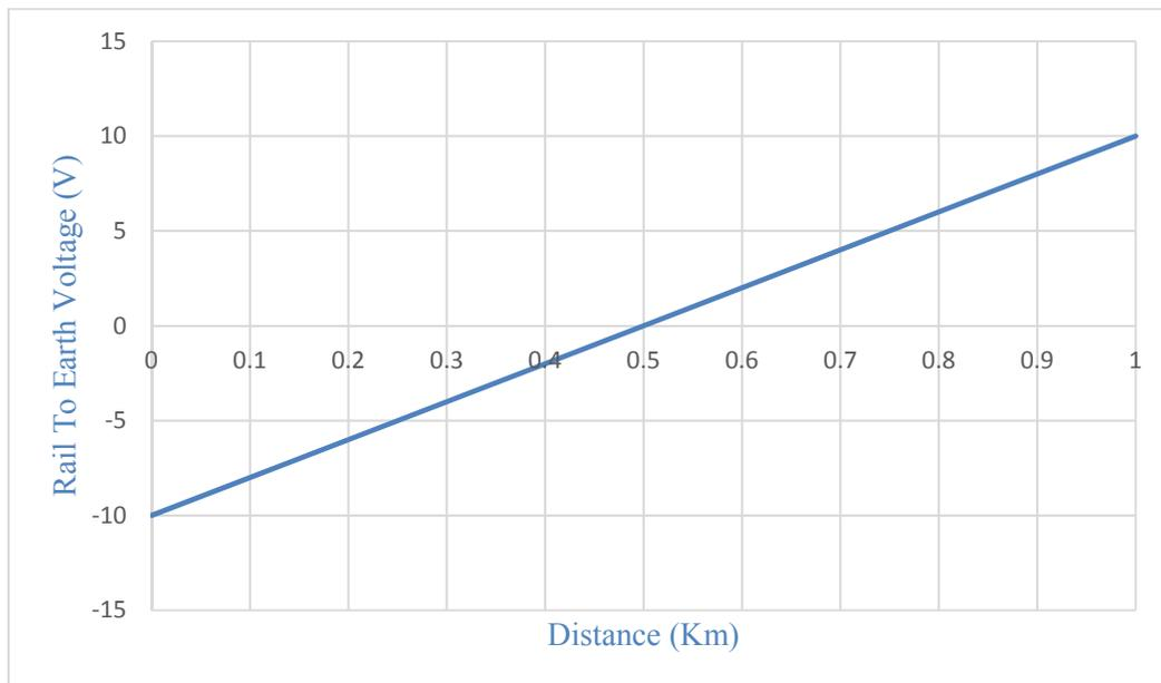
**Figure 46: Rail-to-Earth Voltage for Floating Earthing System**
