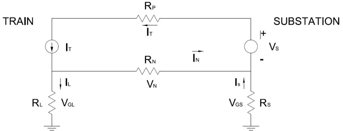
**Figure 2: Simple Circuit Model illustrating Stray Current Components [17]**
