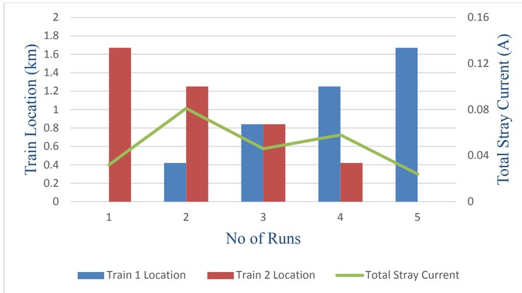
**Figure 62: Total Stray Current with Respect to Varying Train Locations**
