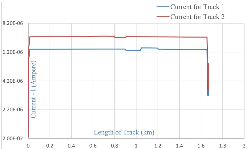
**Figure 59: Maximum Stray Current for Two Track System**
