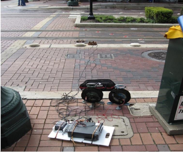
**Figure 33: Track Slab Current Flow Test**
