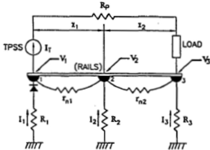
**Figure 14: Basic Stray Current Model using Spherical Electrodes [17]**
