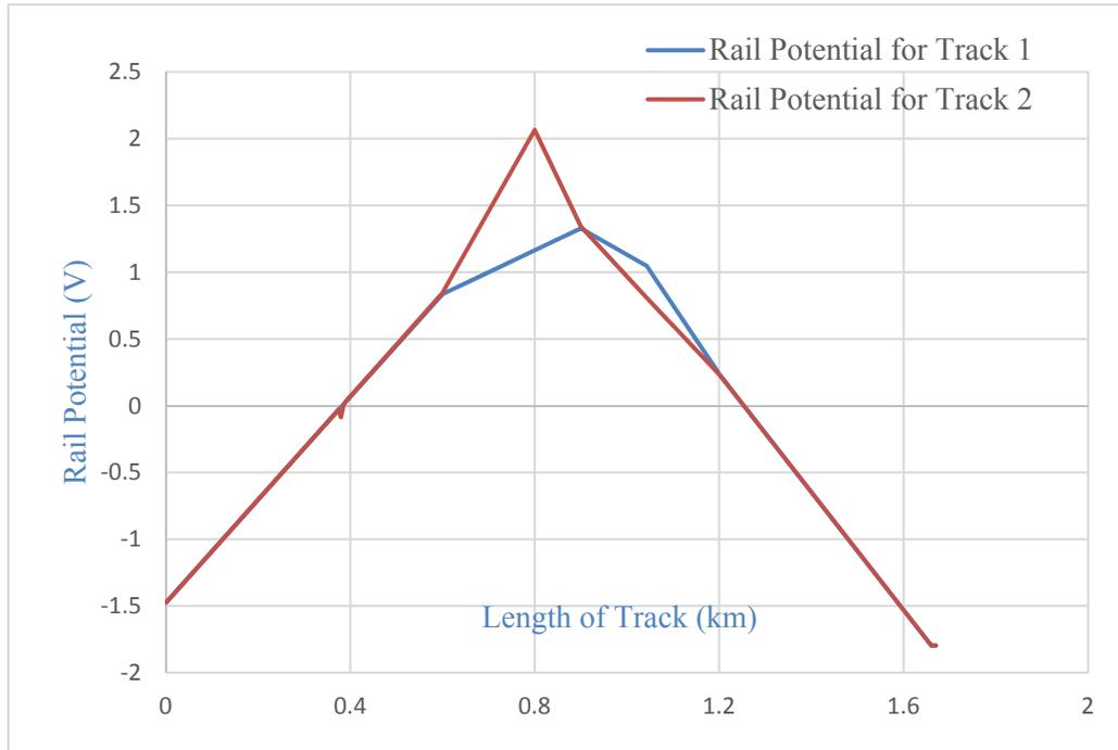
**Figure 60: Rail Potential for the Transit System with Rail Resistivity  $0.06\Omega/\text{km}$**
