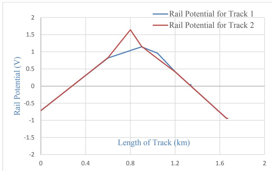
**Figure 63: Rail Potential for Two Track Transit System**
