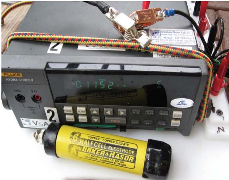
**Figure 31: Fluke Model 2635A Hydra Data Bucket**
