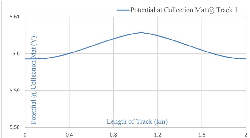
**Figure 54: Potential on Collection Mat with no Cross Bonding**
