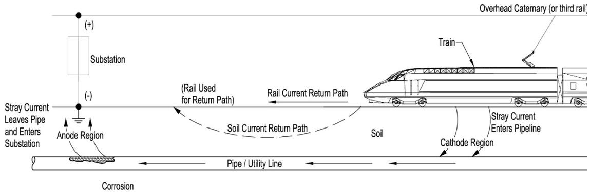
**Figure 1: Stray Current Corrosion Path**
