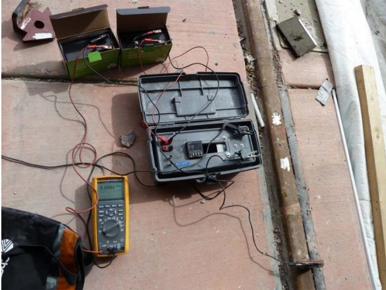
**Figure 38: Track-to-Earth Measurement – Embedded Track**
