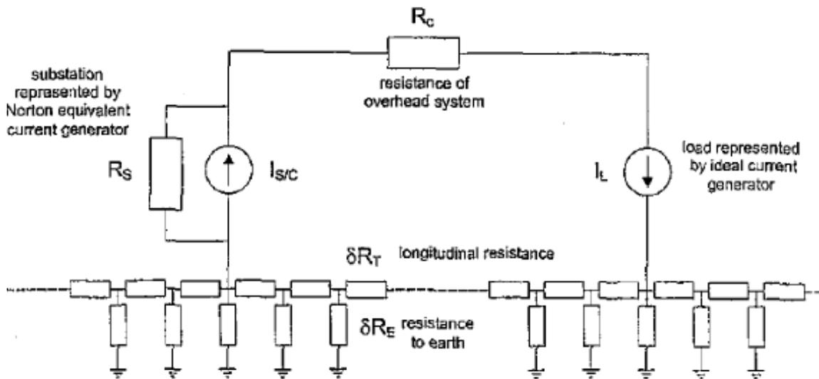
**Figure 12: Equivalent Circuit Representation Using Track “Cells” [33]**
