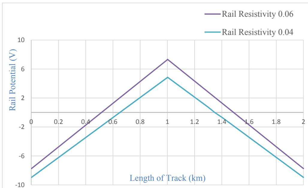
**Figure 51:** Effect of Rail Resistivity on Rail Potential in a Floating System
