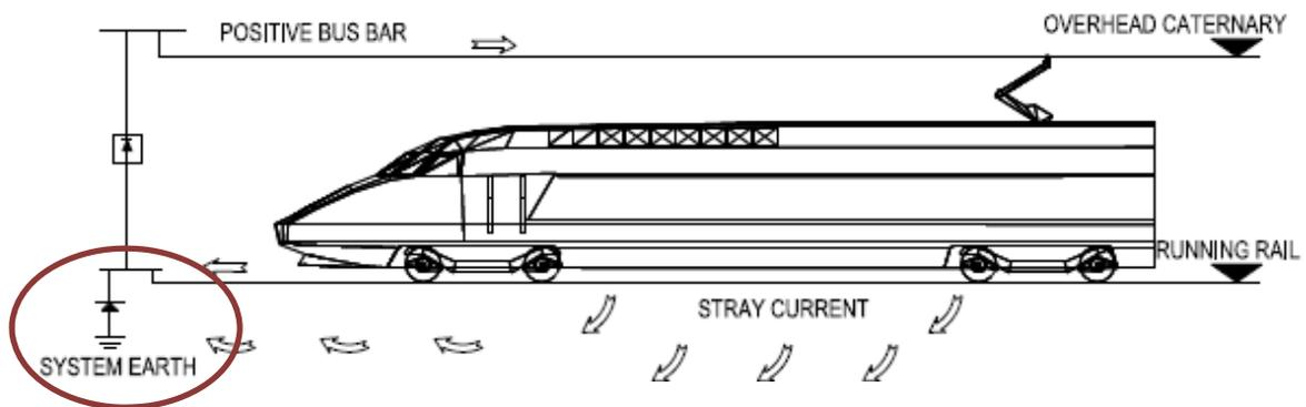
Figure 5: Diode Bonded System
