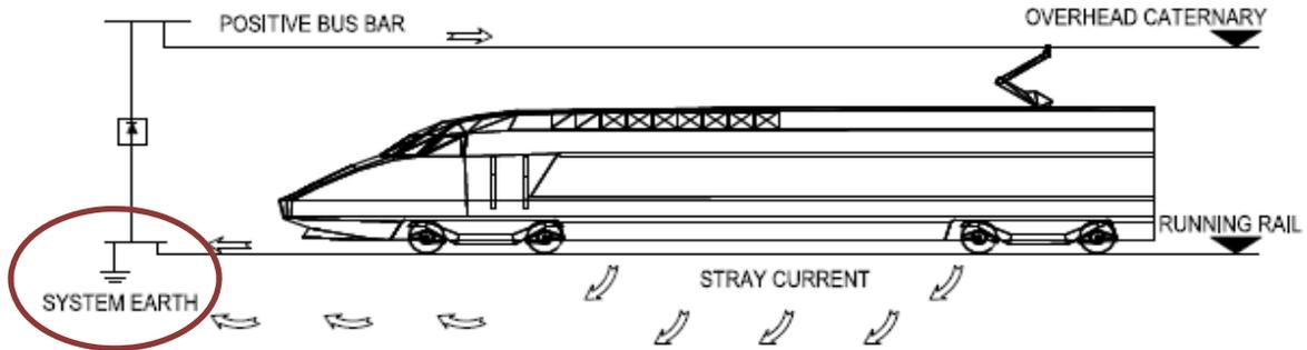
**Figure 3: Grounded / Solidly Bonded System**
