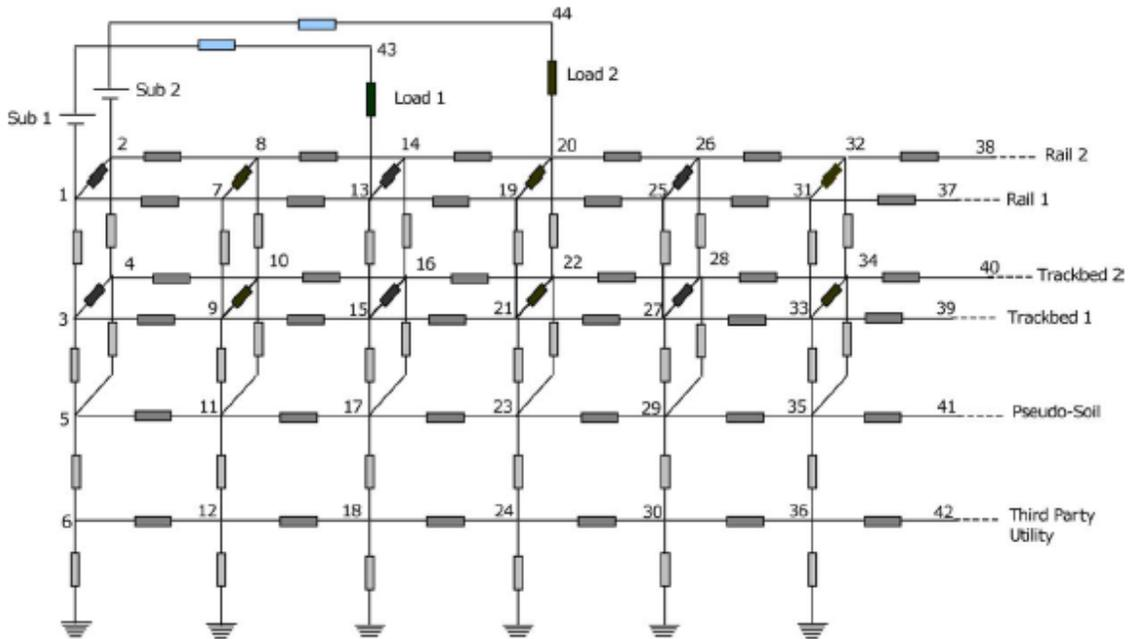
**Figure 16: Resistive Type Network for the Double Track Floating System [39]**
