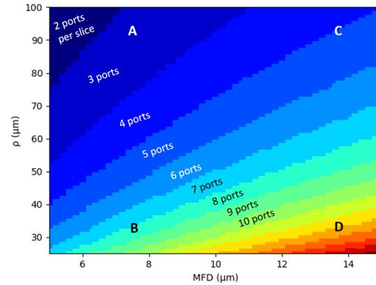
Fig. 12. One dimensional port count dependence on the two principal parameters of the fiber design: MFD and the distance from the outer most core to the fiber center,  $\rho$ . Port counts are calculated assuming that the optimal  $f_1/f_2$  values are used for each design and a maximum actuator angle of 10 degrees.
