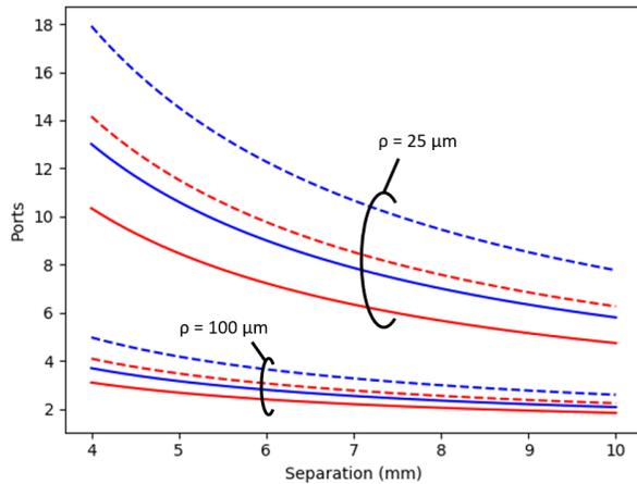
Fig. 6. Maximum number of ports in a single dimension as a function of the port separation, with maximum actuator angle set to 10 degrees. Dashed lines indicate a MFD of  $12\ \mu\text{m}$ , solid lines indicate a MFD of  $8\ \mu\text{m}$ . Red lines are wavelength of  $1620\ \text{nm}$ , blue lines are  $1260\ \text{nm}$ .  $\rho$  is the distance from the outer most core to the fiber center.
