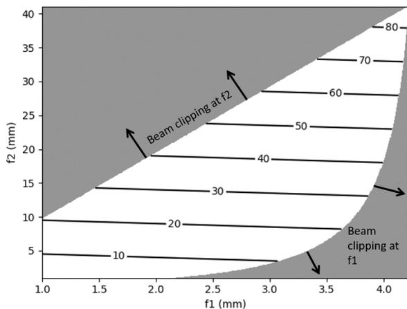
Fig. 4.  $z_2$  (mm) as a function of  $f_1$  and  $f_2$ . The maximum value of  $z_2$  occurs at the maximum possible values of  $f_1$  and  $f_2$  which are in turn restricted by the beam clipping at their respective lenses.
