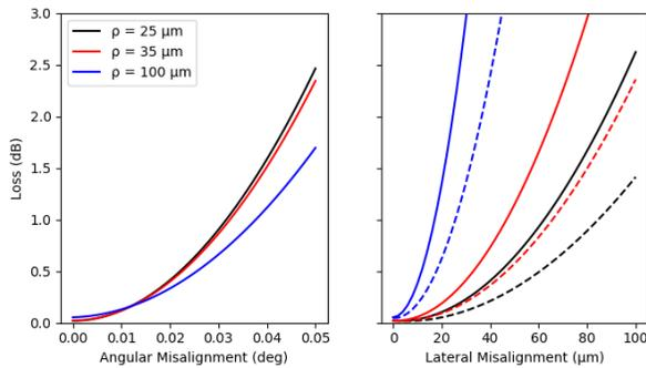
Fig. 8. Estimated total losses across all cores resulting from both angular and lateral misalignment between the collimator and lens array, for  $\rho = 25 \mu\text{m}$ ,  $35 \mu\text{m}$ ,  $100 \mu\text{m}$ . Dashed lines indicate a MFD of  $12 \mu\text{m}$ , solid lines indicate a MFD of  $8 \mu\text{m}$ . The maximum actuator angle is 10 degrees and the loss is wavelength independent.
