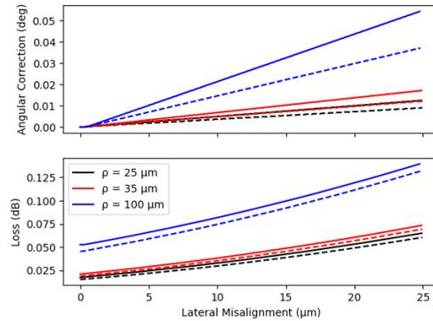
Fig. 9. Required angular correction to compensate for a given lateral misalignment at the collimator, for  $\rho = 25 \mu\text{m}$ ,  $35 \mu\text{m}$ ,  $100 \mu\text{m}$ . Dashed lines indicate a MFD of  $12 \mu\text{m}$ , solid lines indicate a MFD of  $8 \mu\text{m}$ . The maximum actuator angle is 10 degrees and the loss is wavelength independent.
