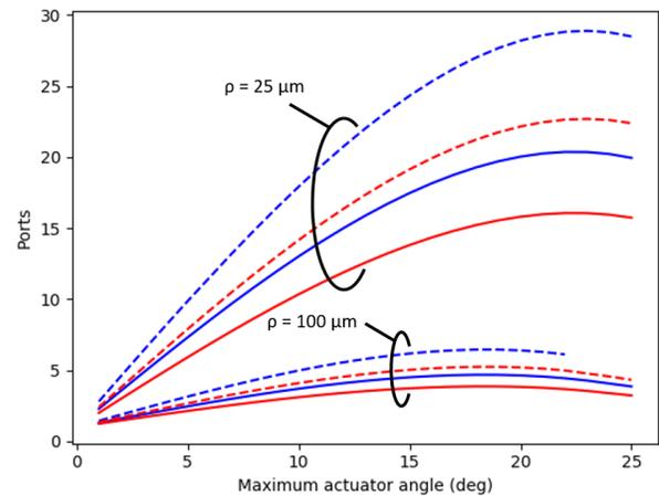
Fig. 5. Maximum number of ports in a single dimension as a function of the maximum actuator angle, with port spacing of 4mm. The  $f_1/f_2$  values are optimized for each angle. Dashed lines indicate a MFD of 12  $\mu\text{m}$ , solid lines indicate a MFD of 8  $\mu\text{m}$ . Red lines are wavelength of 1620 nm, blue lines are 1260 nm.  $\rho$  is the distance from the outer most core to the fiber center.
