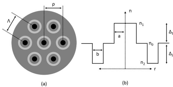
Fig. 11. (a) 7 core hexagonal TA-MCF, with core pitch,  $\Delta$ , and distance from the outer most core to the fiber center,  $\rho$ . (b) Refractive index profile of a trench assisted core,  $n_0$  is the cladding refractive index, with the core and trench index raised and lowered to  $n_1$  and  $n_2$  respectively.
