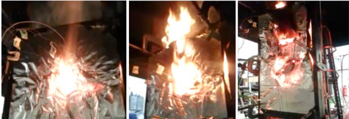
Figure 6. Evolution of the back face of the foam A board tested at 65 \text{ kW}\cdot\text{m}^{-2} at 100-110 min, with smouldering/flaming breaking through.
