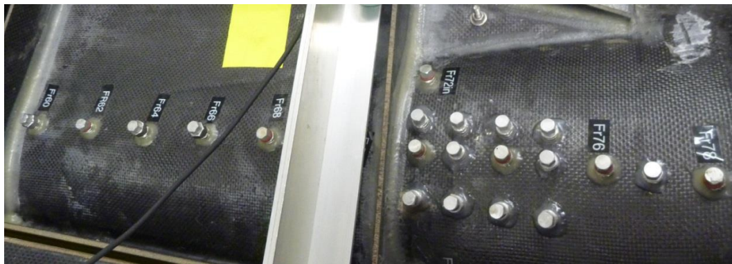
Figure 4 Embedded fitting plugs manufactured on the starboard side of the CB segment
