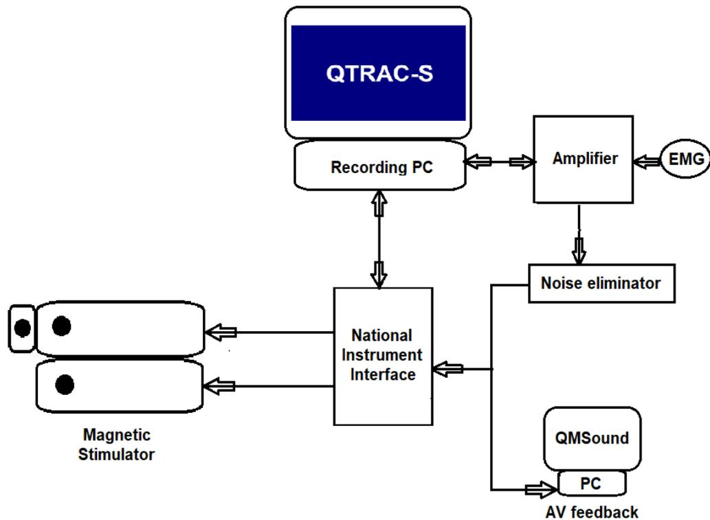
**Figure 2.1. Schematic illustration of the hardware setup.** Magnetic stimulation (intensity and triggering) is controlled by QtracS software. National Instrument Interface consists of a data acquisition card and a shielded connector block. PC – personal computer, AV – audiovisual feedback; EMG – surface electromyography. For details of the equipment, see text. A more detailed description of connections is presented in Appendix A
