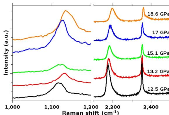
FIG. 1. Unprocessed Raman spectra of vibrational modes of CD<sub>4</sub> of a sample rested at 7 GPa for several days prior to sudden compression to 12.5 GPa (labeled “1st MB” throughout the text).
