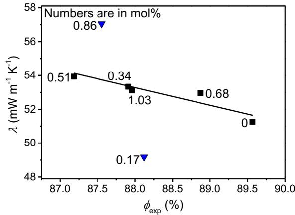
**Fig. 3.** Change in thermal conductivity ( $\lambda$ ) with the porosity ( $\phi_{\text{exp}}$ ). The labels refer to the  $\text{K}_3\text{PO}_4$  content. Outliers are marked with triangles. The errors are smaller than the symbols. The line is a visual guideline.
