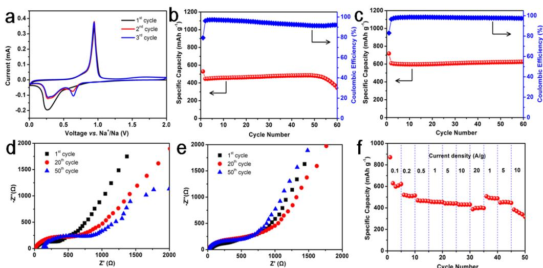
**Fig. 4** a) Cyclic voltammety of A-Sb NRs electrode at a scan rate of  $0.5 \text{ mV s}^{-1}$  between 0.01 to 2.0 V (vs.  $\text{Na}^+/\text{Na}$ ). Cycling performance of b) A-Sb NRs and c) S-Sb NRs at a current density of  $1 \text{ A g}^{-1}$ . Nyquist plots of d) A-Sb NRs and e) S-Sb NRs at discharge state (0.01 V) from 1 MHz to 10 mHz. f) Rate performance of A-Sb NRs electrode at various current densities from 0.1 to  $20 \text{ A g}^{-1}$ .
