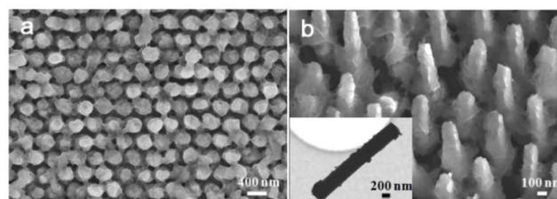
**Fig. 5** SEM images of a) top view and b) tilted view of Sb nanorod arrays electrode after 70 cycles at a current density of  $10 \text{ A g}^{-1}$ . (Inset: TEM image of a single Sb nanorod.)
