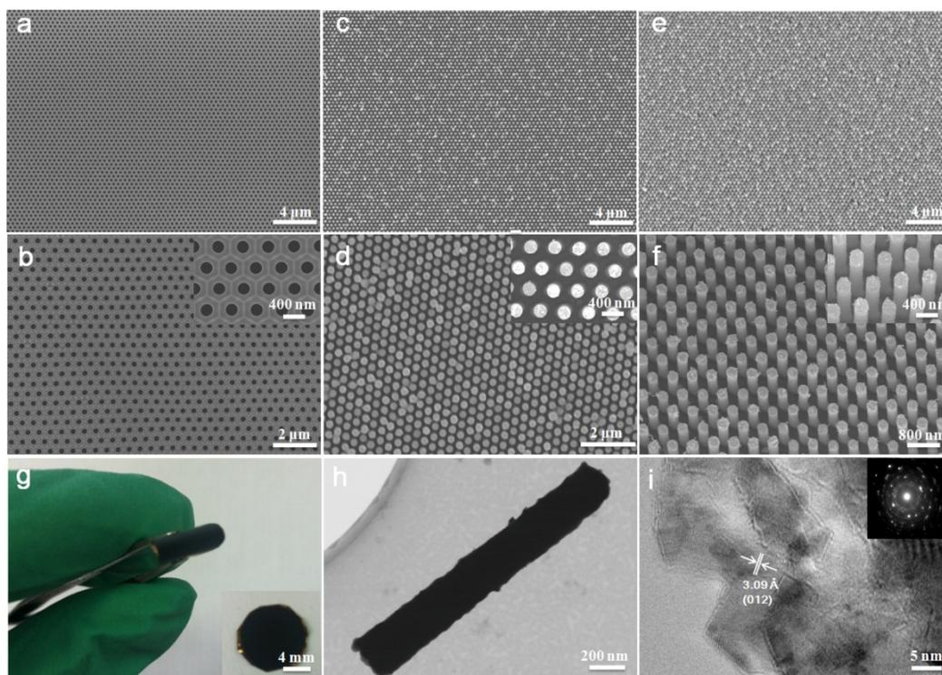
**Fig.1** SEM images of nanoimprinted AAO template (a, b), top view (c, d) and tilted view (e, f) of Sb nanorod arrays. g) Optical image of Sb nanorod arrays on Au/Ni substrate. h) TEM image of a single Sb nanorod. i) HRTEM image of Sb nanorods and SAED pattern (inset).
