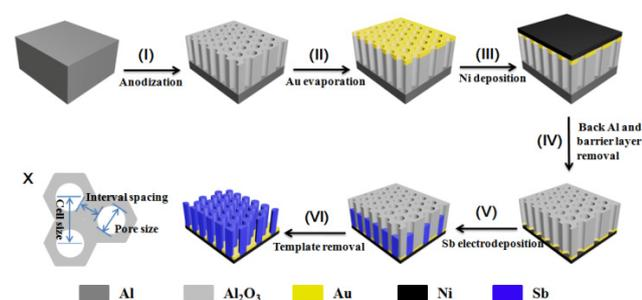
**Scheme 1** Schematic illustration of the fabrication processes of Sb nanorod arrays by using the nanoimprinted AAO templating technique with the assistance of an electrodeposition process. X) Size schematic of AAO template.
