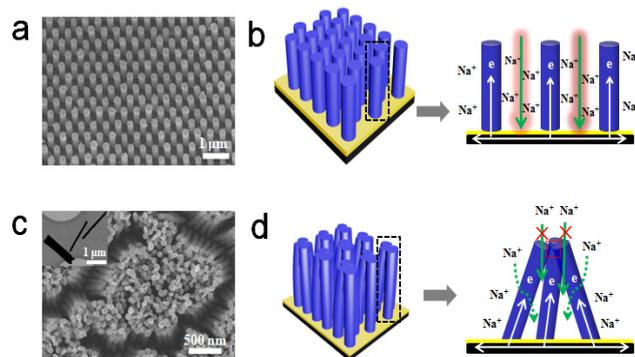
**Fig. 3** SEM images of a) S-Sb NRs and c) A-Sb NRs (Inset: TEM image of A-Sb NRs). Corresponding schematic illustration of transport mechanism of Na ions and electrons in b) S-Sb NRs and d) A-Sb NRs.
