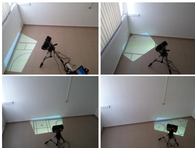
Fig. 1. Overview of the system in a proof-of-concept experiment of a bathroom layout projected on the floor. The system is composed of a laser scanner to localize itself in the room; an angled projector then projects the relevant information on the construction surface. When the system is moved to a new location, it automatically re-localizes itself in seconds and projects the accurate and updated design information. The system is first calibrated to calculate how to pre-warp the image in order for the image to be precisely projected on the
