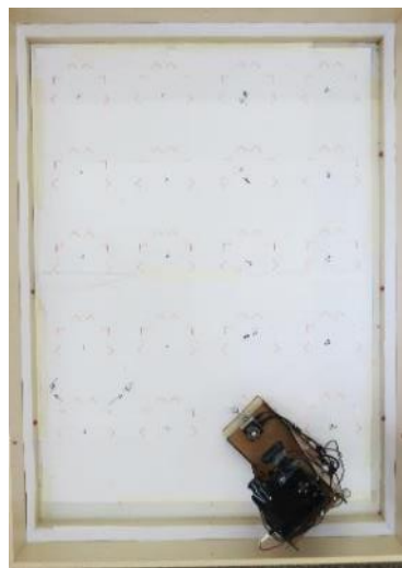
Fig. 5. Localization verification experiment. Experiment for testing the localization algorithm. Sixty measurements were conducted in a 1 m x 1.4 m room mockup. Four poses in the x-direction, five poses in the y-direction, and three orientations ( -45^\circ , 0^\circ , 45^\circ ).
