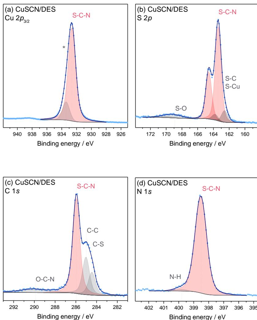
**Figure S8.** Peak fit analysis of the core level spectra measured for CuSCN layers processed from CuSCN/DES including: (a) Cu  $2p_{3/2}$ , (b) S  $2p$ , (c) C  $1s$ , and (d) N  $1s$ .
