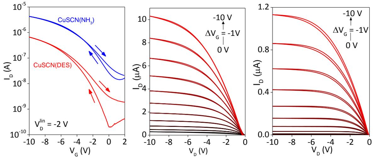
**Figure S13.** Electrical characteristics of TG-BC CuSCN TFTs based on P(VDF-TrFE-CFE) polymer as the gate dielectric. The TFT channel dimensions employed are  $L = 30 \mu\text{m}$  and  $W = 1000 \mu\text{m}$ . (left) Transfer characteristics measured in the linear regime. Output characteristics of CuSCN TFTs processed from NH<sub>3</sub>(aq) (middle), and DES (right).
