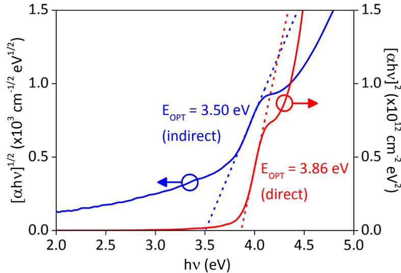
**Figure S3.** Plots of  $(\alpha h\nu)^2$  and  $(\alpha h\nu)^{1/2}$  calculated from absorbance measurements of an ammonia-processed CuSCN layer spin-cast on quartz from a CuO/NH<sub>4</sub>SCN precursor formulation. From the linear regions of the plots an indirect bandgap of 3.50 ( $\pm 0.05$ ) eV and a direct bandgap of 3.86 ( $\pm 0.05$ ) eV, were extracted.
