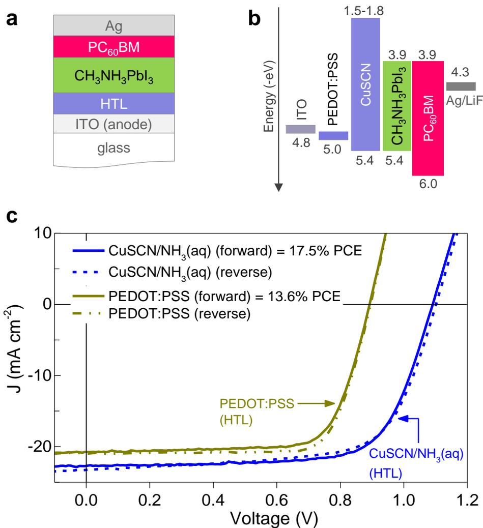
**Figure 6.** (a) Schematic cross-section of the cell architecture employed, and (b) corresponding material energetics. (c) J-V characteristics measured under simulated solar illumination for two CH<sub>3</sub>NH<sub>3</sub>PbI<sub>3</sub> solar cells based on CuSCN/NH<sub>3</sub>(aq) and PEDOT:PSS HTLs.
