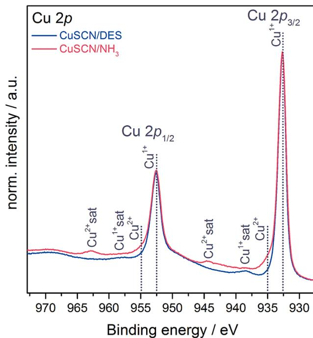
**Figure S10.** Cu 2p core level spectra of CuSCN layers processed from CuSCN/DES and CuSCN/NH<sub>3</sub>(aq) solutions including satellite structures.
