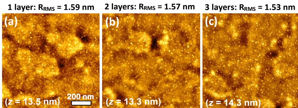
**Figure S4.** Topography AFM images (scan area of 1  $\mu\text{m}^2$ ) of ammonia-processed CuSCN HTLs deposited on glass/ITO. (a) The CuSCN layer was spin-cast at 2000 rpm from a 15 mg ml<sup>-1</sup> CuSCN precursor solution and annealed at 100 °C. (b) and (c) show the topography images of CuSCN layers formed after 2 and 3, respectively, sequential spin-casting rounds of CuSCN using the same growth conditions. In all images, lighter colours correspond to higher regions
