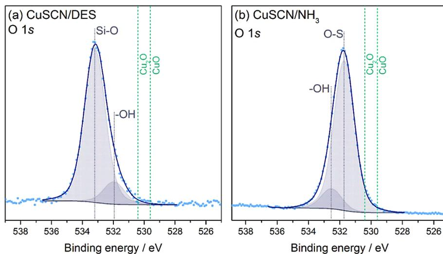
**Figure S11.** Peak fit analysis of the O 1s core level spectra of; (a) CuSCN/DES and (b) CuSCN/NH<sub>3</sub>(aq).
