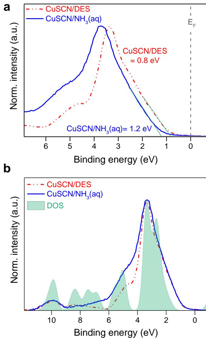
**Figure 3.** (a) Valence band spectra of CuSCN/DES and CuSCN/NH<sub>3</sub>(aq) layers where the position of the VB<sub>max</sub> with respect to E<sub>F</sub> is also shown. (b) Experiment and one electron cross section corrected density of states (DOS) for CuSCN/DES and CuSCN/NH<sub>3</sub>(aq) layers from DFT calculations. In (b) the data sets from (a) are aligned to the position of the Cu 3d contribution of CuSCN/DES.
