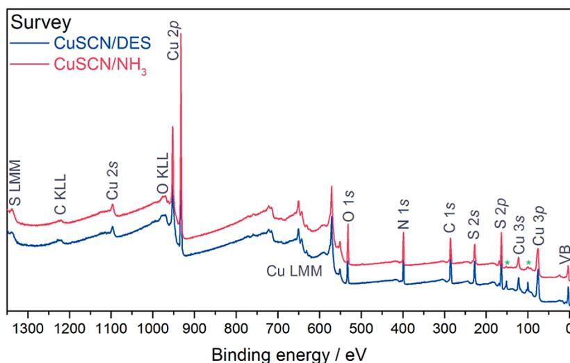
**Figure S7.** Survey spectra of CuSCN/DES and CuSCN/NH<sub>3</sub> indicating core levels and Auger lines. The lines at 100 and 150 eV, marked with an asterisk, correspond to the Si 2*p* and 2*s* core lines of the substrate.
