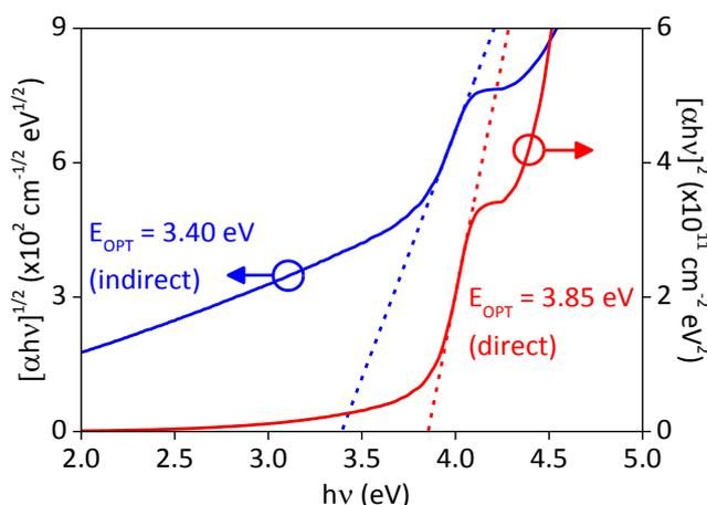
**Figure S1.** Plots of  $(\alpha h\nu)^2$  and  $(\alpha h\nu)^{1/2}$  calculated from absorbance measurements of a DES-processed CuSCN layer on quartz. The linear regions correspond to an indirect bandgap of 3.40 ( $\pm 0.05$ ) eV and a direct bandgap of 3.85 ( $\pm 0.05$ ) eV.
