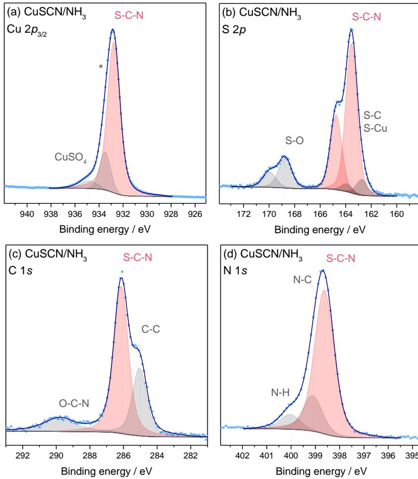
**Figure S9.** Peak fit analysis of the core level spectra measured for CuSCN layers processed from CuSCN/NH<sub>3</sub>(aq) including: (a) Cu  $2p_{3/2}$ , (b) S  $2p$ , (c) C  $1s$ , and (d) N  $1s$ .
