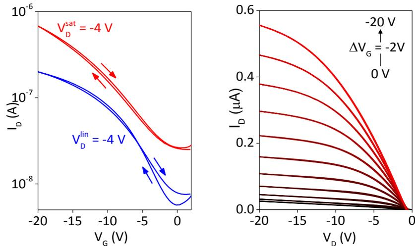
**Figure S14.** Electrical characterization of a TG-BC CuSCN-based TFT with a P(VDF-TrFE-CFE) polymer dielectric, which has channel dimensions of  $L = 30 \mu\text{m}$  and  $W = 1000 \mu\text{m}$ . Transfer (Left) and output (right) characteristics of a CuSCN TFT processed from an aqueous CuO/NH<sub>4</sub>SCN precursor solution.
