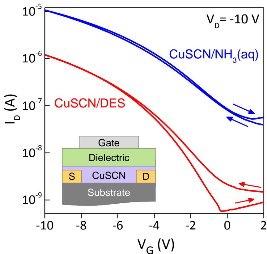
**Figure 4.** Transfer characteristics of a CuSCN TFT processed via spin-casting from a  $\text{CuSCN}/\text{NH}_3(\text{aq})$  solution. Inset shows a schematic of the staggered TG-BC transistor architecture employed with Au S-D contacts and Al gate electrode. The channel dimensions of the transistor are  $L = 30 \mu\text{m}$  and  $W = 1000 \mu\text{m}$ .
