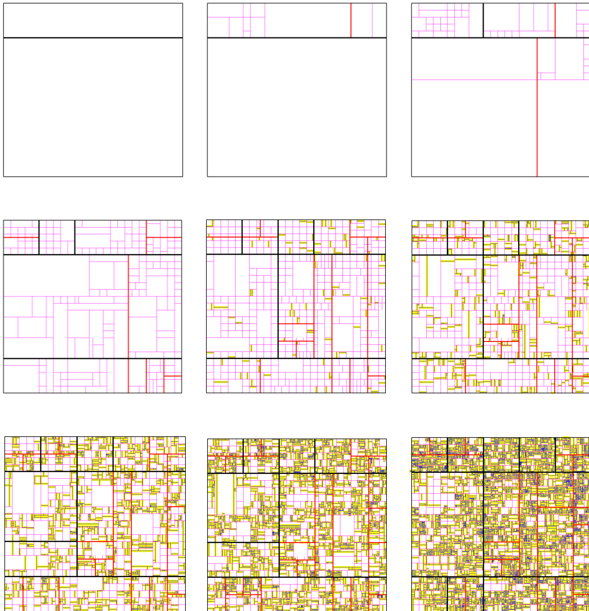
Figure 1: NetStoat simulation of the generation of a street network. This shows the network at nine stages of growth, after 1, 10, 50, 200, 600, 1000, 2000, 4000 and 8000 iterations
