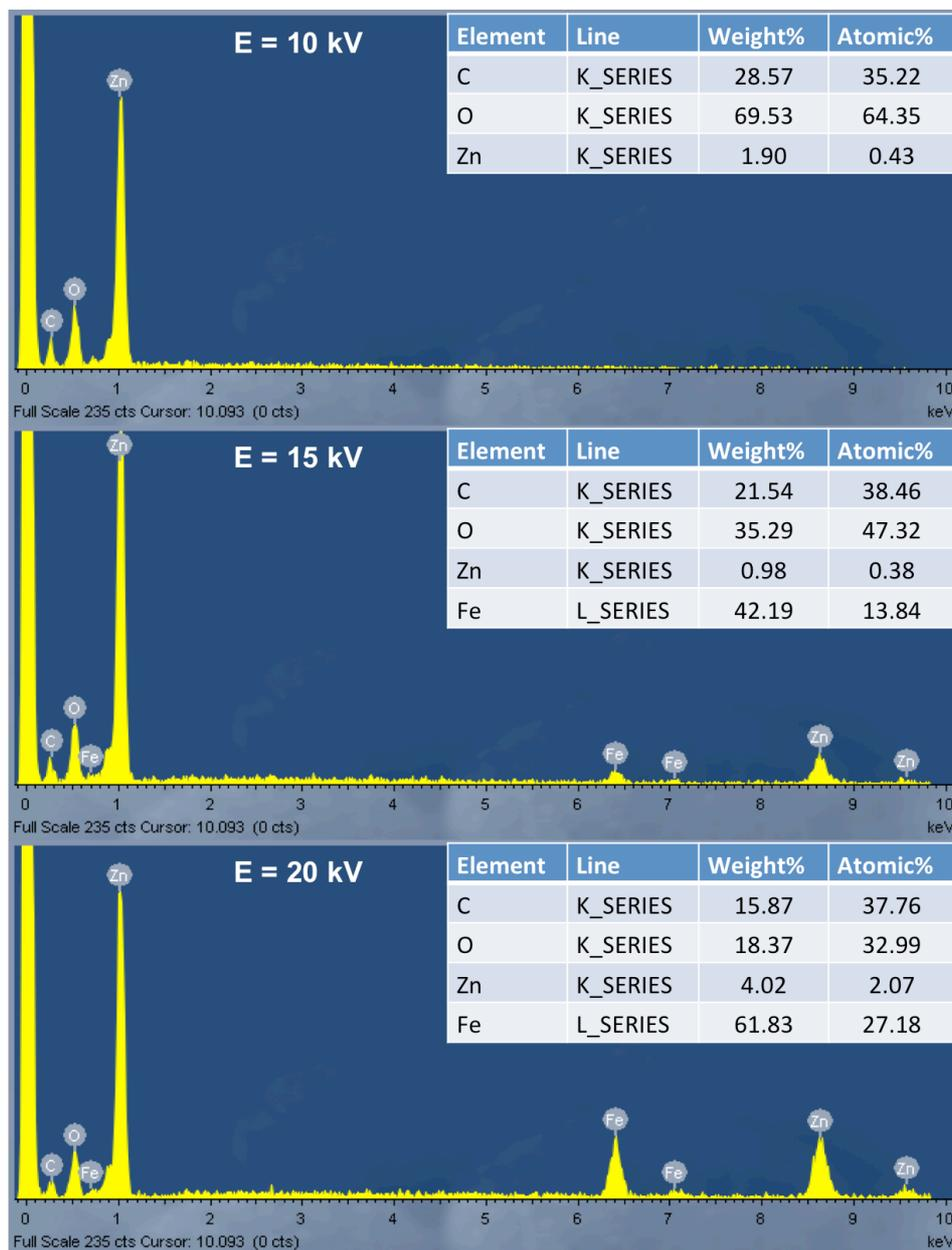
**Fig. S2.** EDS spectra of the heterojunction  $\alpha$ -Fe<sub>2</sub>O<sub>3</sub>/ZnO film with the use of different accelerating energy of 10 kV, 15 kV and 20 kV. The inset tables give details about weight% and atomic% of all elements detected.
