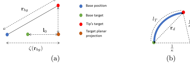
Fig. 4. (a) The base (blue dot) will be forced to move to a target position (green dot) located at a distance l_0 from the projection (orange dot) of the goal position (red dot). (b) The length of the manipulator will be forced to reach a target length l_T , i.e. the curve length from the target base position (green dot) to the goal position (red dot).
