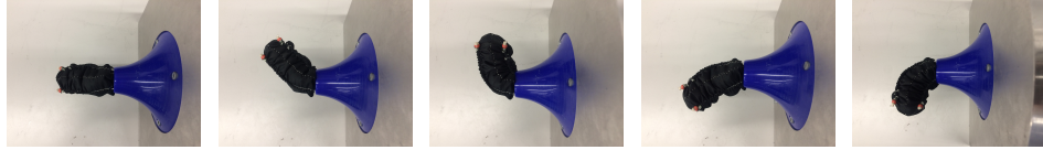
Fig. 2. The manoeuvrability of the soft, inflatable manipulator.
